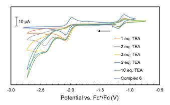
Fig. 7 Cyclic voltammograms of complex 6 (1 mM) with the addition of 1–10 mM of TEA in THF/[Bu<sub>4</sub>N]PF<sub>6</sub> (scan rate = 0.1 V s<sup>-1</sup>); the arrow indicates the scan direction.
