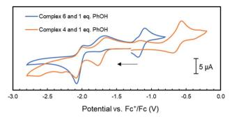
Fig. 6 Cyclic voltammograms of complex 4 and 6 (1 mM) with the addition 1 mM of phenol in THF/[Bu<sub>4</sub>N]PF<sub>6</sub> (scan rate =  $0.1 \text{ V s}^{-1}$ ); the arrow indicates the scan direction.
