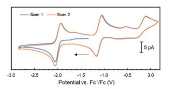
Fig. 5 Cyclic voltammograms of complex 6 (1 mM) in THF/[Bu<sub>4</sub>N]PF<sub>6</sub> (scan rate =  $0.1 \text{ V s}^{-1}$ ); the arrow indicates the scan direction.
