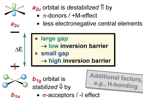
**Fig. 7** Simplified presentation of the factors that determine the height of the planar inversion barrier of tetrahedral p-block element-based species, for which the substituents are more electronegative than the central elements.
