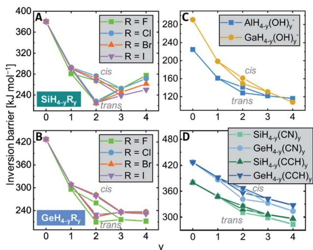
Fig. 4 Additive substituent effects for the inversion barrier of (A) SiH<sub>4-y</sub>R<sub>y</sub>, (B) GeH<sub>4-y</sub>R<sub>y</sub>, with R = F, Cl, Br, I, of (C) AlH<sub>4-y</sub>(OH)<sub>y</sub><sup>-</sup> and GaH<sub>4-y</sub>(OH)<sub>y</sub><sup>-</sup>, and of (D) EH<sub>4-y</sub>R<sub>y</sub>, with E = Si, Ge and R = CN, CCH.
