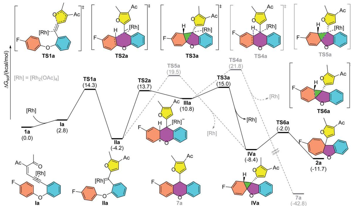
Scheme 2 Free energy profiles of  $\text{Rh}_2(\text{II})$ -catalyzed reaction pathways of enynone **1a**. If not otherwise noted, relative Gibbs free energies computed at the M06/def2TZVP-SMD(dichloroethane)//B3LYP-D3(BJ)/def2SVP theoretical level are reported in  $\text{kcal mol}^{-1}$ .
