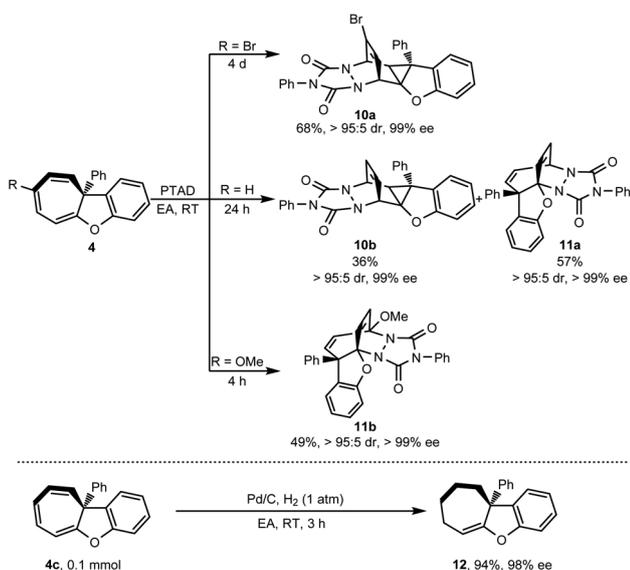
Scheme 6 Transformation of cycloheptatriene **4**.<sup>a</sup> The reaction was conducted on 0.1 mmol scale, PTAD (1.05 equivalent).
