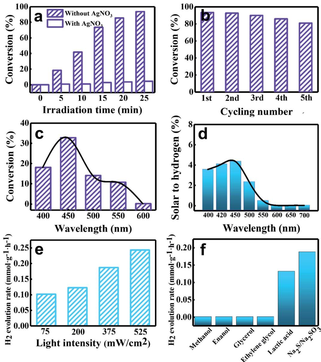
Fig. 4 (a) Photoactivities of ZPM towards 4-NA reduction with and without addition of AgNO<sub>3</sub> as an electron scavenger; (b) cycling reactions of ZPM; (c) action spectrum for photoreduction of 4-NA over ZPM under different monochromatic light irradiation; (d) S.T.H conversion efficiency of ZPM under monochromatic light irradiation; photocatalytic hydrogen evolution rates of ZPM (e) under different light intensities and (f) utilizing different sacrificial reagents.
