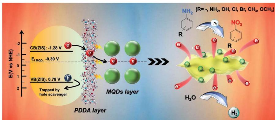
Scheme 1 Schematic illustration of the photocatalytic mechanism of ZPM.
