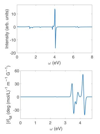
Fig. 11 Upper panel: circular dichroism spectrum eqn (9) of polaritons with  $\delta=0$ ,  $g=1.028\times 10^{-1}$  V Å $^{-1}$  excited by linearly polarized pulse. Lower panel: magnetic circular dichroism of Mg-porphyrin molecule in the magnetic field of 8 T (or 3.403 5  $\times$  10 $^{-5}$  a.u.).
