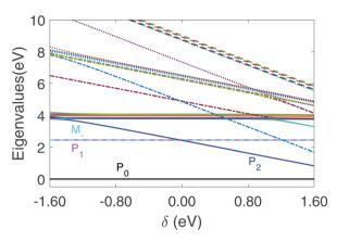
Fig. 13 Polariton energy variation with detuning for coupling strength  $g=1.028\times 10^{-1}$  V Å $^{-1}$ . We mark  $|P_0\rangle$ ,  $|P_1\rangle$ ,  $|P_2\rangle$ ,  $|M_-\rangle$  with color. The legend of other polariton states are given in Fig. S1 in ESI.†
