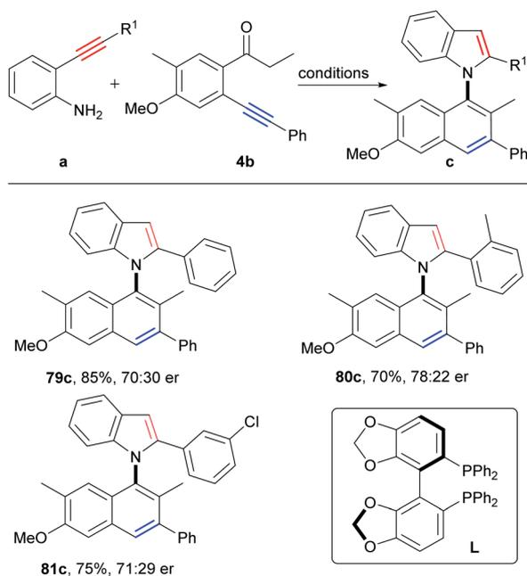
Scheme 7 Substrate scope of axially chiral compounds. Reaction conditions: (1) **a** (0.2 mmol), **4b** (1.2 equiv.), CuI (5 mol%), Cs<sub>2</sub>CO<sub>3</sub> (2.0 equiv.) HFIP, 80 °C, 50 min; (2) PdCl<sub>2</sub> (5 mol%), L (6 mol%) HFIP, 80 °C, 15 h.
