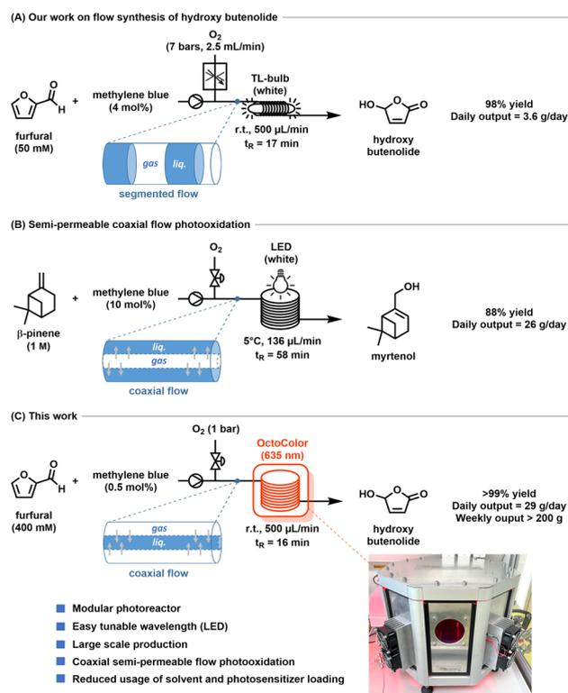
Fig. 1 A. Our segmented flow design for the photooxidation of furfural. B. Previously described coaxial flow design for the photooxidation of  $\beta$ -pinene; with liquid phase on outside. C. Coaxial flow photooxidation of furfural using the modular photoreactor OctoColor; with liquid phase on inside for convenience.
