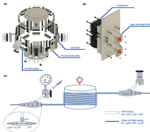
Fig. 2 A. Schematic exploded view of OctoColor reactor. B. Schematic exploded view of LED plate. For details of construction, see SI OctoColor construction manual. C. Schematic representation of a coaxial flow reactor.
