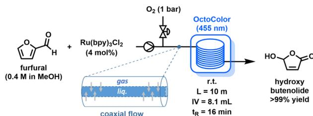
Fig. 3 Photooxidation of furfural towards hydroxybutenolide using Ru(bpy)<sub>3</sub>Cl<sub>2</sub> as photosensitizer. OctoColor arranged with blue LED plates. Reaction conditions in coaxial semi-permeable flow: 0.4 M furfural in methanol, Ru(bpy)<sub>3</sub>Cl<sub>2</sub> (4 mol%), rt, oxygen, 455 nm, 8.1 mL internal volume.
