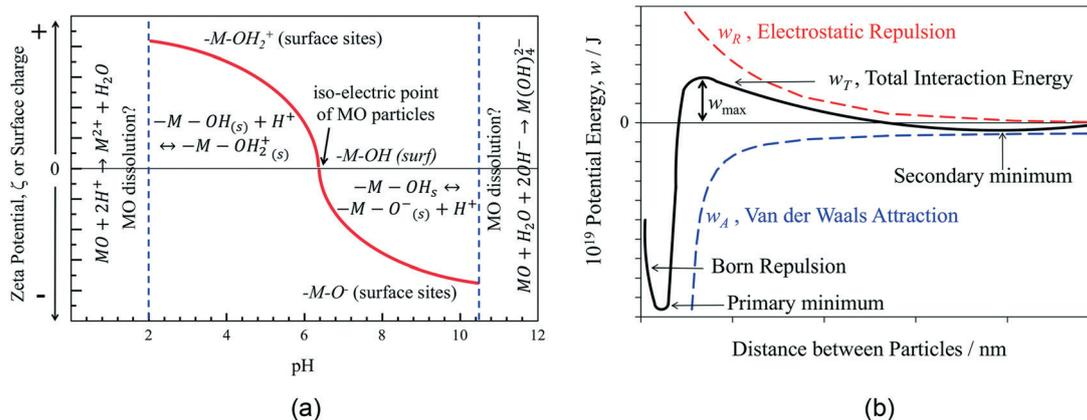
Fig. 10 (a) Schematic pH effect on surface charge and hence zeta potential on metal oxide particles. (b) Schematic effect of inter-particle separation on electrostatic repulsion ( $w_R$ ), van der Waals attraction ( $w_A$ ), and total ( $w_T = w_R + w_A$ ) interaction potentials.
