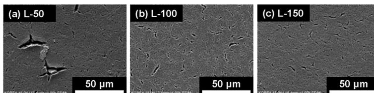
Fig. 19 Cracking in the sintered LSCF layers at a luminosity setting of 50 (a), 100 (b), and 150 (c). Reproduced with permission.<sup>85</sup>
