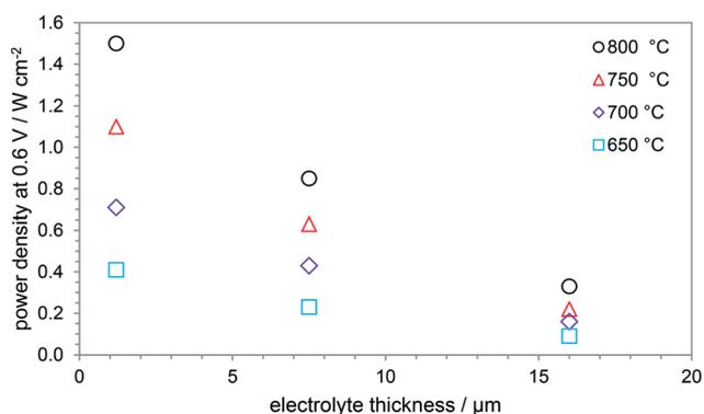
Fig. 24 Effect of electrolyte thickness on power densities at 0.6 V applied potential difference for 650–750 °C.<sup>80,83,101</sup>
