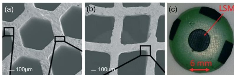
Fig. 22 (a) Hexagonal, and (b) square CGO microstructures of 12  $\mu\text{m}$  depth each, comprising 20 printed layers. Reproduced with permission.<sup>88</sup> (c) photograph of the printed LSM deposited using aqueous-based ink.
