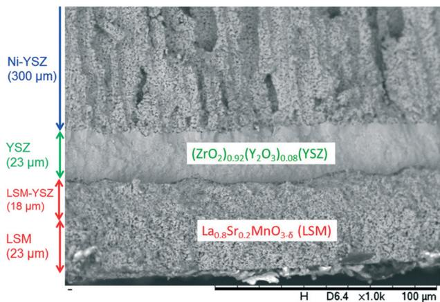
Fig. 16 SEM image of cross-sectional structure of LSM|LSM–YSZ|YSZ|Ni–YSZ SOFC with electrolyte fabricated by inkjet printing.<sup>81</sup>
