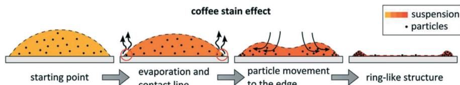
Fig. 13 Schematic of formation of ring-like structure at the boundary of droplets in the coffee stain effect (reproduced with permission<sup>70</sup>).
