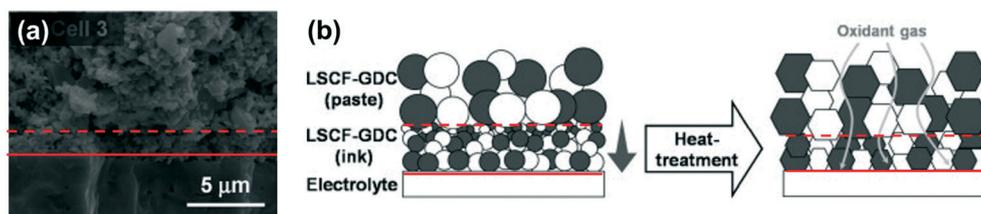
Fig. 26 Graded electrode micro-structure incorporating inkjet printing and conventional pasted electrodes with (a) scanning electron micrograph and (b) schematic. Reproduced with permission.<sup>98</sup>
