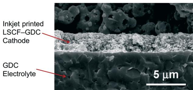
Fig. 21 SEM image of the cross section of the printed cathode layer. Reproduced with permission.<sup>87</sup>
