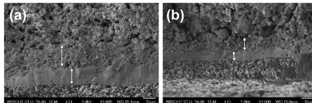
Fig. 17 Cross sectional SEM images of sintered, printed YSZ electrolyte and NiO–YSZ composite layers. (a) Layers produced using NiO particles of  $R = 15$  nm; 12  $\mu\text{m}$  thick electrolyte (top) and composite NiO–YSZ interlayer (bottom). (b) Layers produced using NiO particles of  $R = 150$  nm; 6  $\mu\text{m}$  thick YSZ electrolyte layer and composite NiO–YSZ interlayer. Reproduced with permission.<sup>82</sup>
