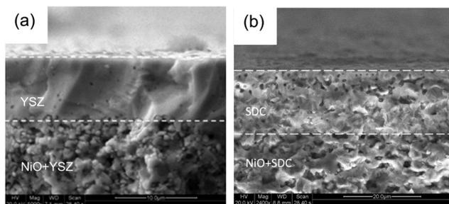
Fig. 23 SEM micrographs showing (a) printed YSZ on Ni-YSZ, and (b) printed SDC on Ni-SDC; post sintering. Reproduced with permission.<sup>90</sup>
