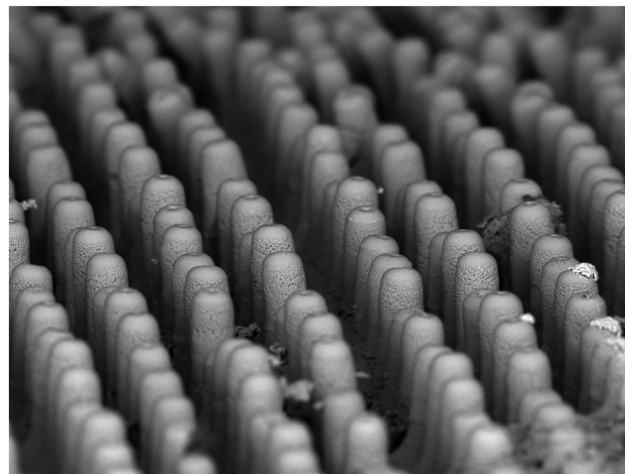
Fig. 27 SEM photomicrograph of pillar array of sintered YSZ overprinted with sintered LSM.
