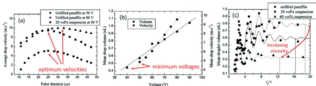
**Fig. 14** (a) Effect of pulse duration on droplet velocity; (b) effect of voltage amplitude on droplet volume and velocity; (c) droplet volume relationship with time/inverse of frequency,  $t_p = f^{-1}$ , for a study with paraffin suspensions, normalised by  $\tau$ , the optimal pulse time,  $P_t$ . Data for paraffin wax jetted at a frequency of 10 kHz and a pulse duration of 30  $\mu$ s. Reproduced with permission.<sup>35</sup>
