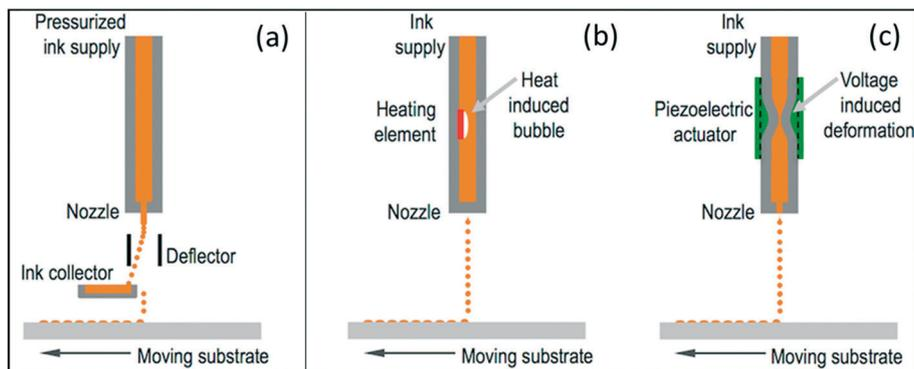
Fig. 3 Schematic representation of (a) continuous inkjet (CIJ) and drop on demand (DOD) inkjet printing systems using (b) thermal and (c) piezoelectric technology (reproduced with permission<sup>33</sup>).
