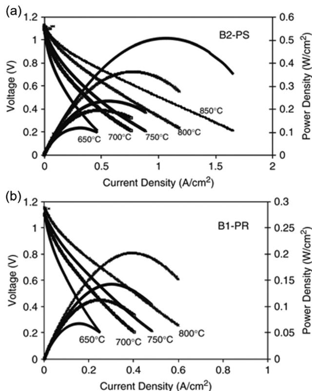
Fig. 25 Effect of current density on cell potential difference for (a) conventional hand-pasted and (b) printed electrode. Reproduced with permission.<sup>83</sup>
