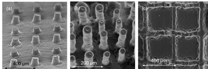
**Fig. 18** (a) 50 and (b) 180 layers of YSZ printed to fabricate micro-pillar arrays; (c) a YSZ square lattice printed onto a NiO-YSZ substrate. Reproduced with permission.<sup>51</sup>
