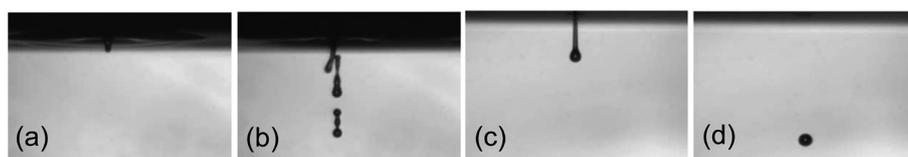
**Fig. 8** Images of droplet ejection and flight for  $Z > 10$  (a and b), and  $1 < Z < 10$  (c and d). Reproduced with permission.<sup>47</sup>
