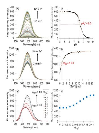
Fig. 2 Emission spectra in water of 14  $\mu$ M 4 as a function of (a) H<sup>+</sup>, (b) Ba<sup>2+</sup> at 10<sup>-4</sup> M H<sup>+</sup>, and (c) methanol/water solvent compositions at 10<sup>-4</sup> M H<sup>+</sup>, and the intensity–concentration profiles.  $\lambda_{ex}=400$  nm.
