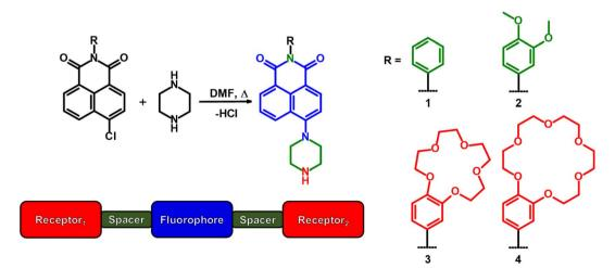
Scheme 1 The synthesis of 4-piperazino-N-aryl-1.8-naphthalimide molecular logic gates 1-4 and the design format of 3 and 4.
