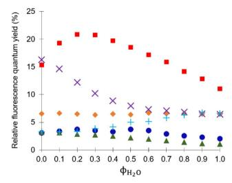
Fig. 4 Fluorescence quantum yields ( $\Phi_{\rm F}$ ) in different water/methanol solvent compositions as a water volume fraction at  $10^{-4}$  M H $^+$  for ( $\bullet$ ) 9  $\mu$ M 1-H $^+$ , ( $\blacktriangle$ ) 10  $\mu$ M 2-H $^+$ , ( $\bullet$ ) 9  $\mu$ M 3-H $^+$ , ( $\star$ ) 9  $\mu$ M 3-H $^+$  and  $10^{-2}$  M Na $^+$ , (+) 14  $\mu$ M 4-H $^+$ , and ( $\blacksquare$ ) 14  $\mu$ M 4-H $^+$  and  $10^{-2}$  M Ba<sup>2+</sup>.
