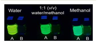
Fig. 1 Molecule 4 irradiated with 365 nm light in water, 1:1 (v/v) water/methanol and methanol with  $10^{-4}$  M H<sup>+</sup> (vials A) and  $10^{-11}$  M H<sup>+</sup> (vials B).
