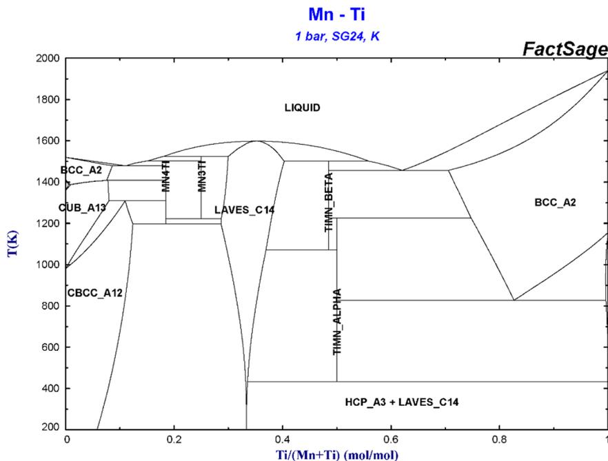
Fig. 2 Binary phase diagram of Mn–Ti.<sup>57,58</sup>
