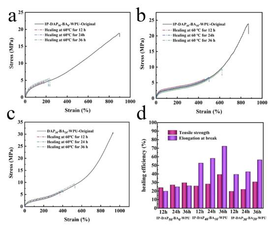
Fig. 6 Original and self-healed tensile stress-strain curves (a-c) and self-healing efficiency (d) of IP-DAP $_{50}$ -BA $_{0}$ -WPU, IP-DAP $_{40}$ -BA $_{10}$ -WPU and IP-DAP $_{30}$ -BA $_{20}$ -WPU films after healing at 60 °C for 12 h, 24 h, and 36 h.
