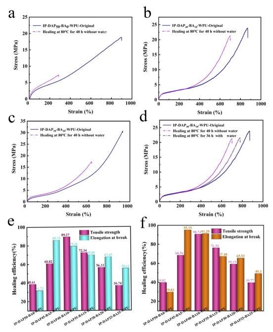
Fig. 7 Original and self-healed tensile stress-strain curves (a-c) of IP-DAP<sub>x</sub>-BA<sub>y</sub>-WPU films after healing at 80 °C for 40 h without water. (d) Representative original and self-healed tensile stress-strain curves of IP-DAP<sub>40</sub>-BA<sub>10</sub>-WPU films under different conditions. (e) Self-healing efficiency of IP-DAP<sub>x</sub>-BA<sub>y</sub>-WPU films healed at 80 °C for 40 h without water and (f) healed at 80 °C for 36 h with the aid of water.
