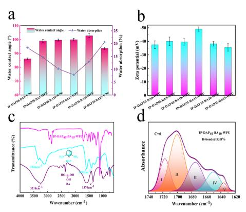
Fig. 2 (a) Water contact angle (WCA) and water absorption (WA) of different IP-DAP $_x$ -BA $_y$ -WPU samples. (b) Zeta potential values of different IP-DAP $_x$ -BA $_y$ -WPU emulsions. (c) FT-IR spectra of BA, DAP and IP-DAP $_{40}$ -BA $_{10}$ -WPU in the frequency range of 650–4000 cm $^{-1}$ . (d) FTIR spectra of IP-DAP $_{40}$ -BA $_{10}$ -WPU in the C=O stretching vibration region.
