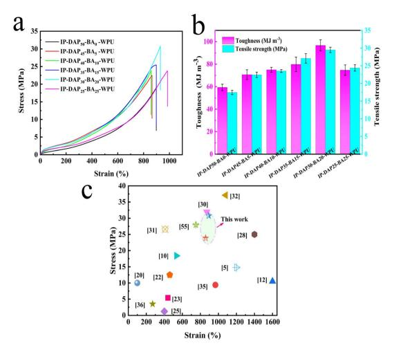
Fig. 4 (a) Stress-strain curves. (b) Tensile strength and toughness of different IP-DAP $_X$ -BA $_y$ -WPU films. (c) Mechanical performance of the representative IP-DAP $_{40}$ -BA $_{10}$ -WPU and IP-DAP $_{30}$ -BA $_{20}$ -WPU films in this work compared with those of other studies.
