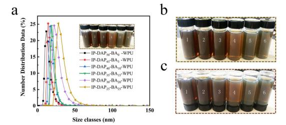
Fig. 1 (a) Particle size and distribution of the as-prepared WPU particles. Color and appearance of IP-DAP<sub>x</sub>-BA<sub>v</sub>-WPU emulsions (b) before and (c) after centrifugation in natural light.
