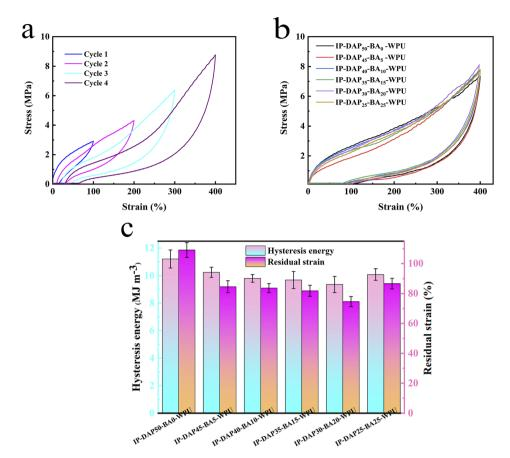
Fig. 5 (a) Sequential cyclic tensile curves of the IP-DAP<sub>30</sub>-BA<sub>20</sub>-WPU film at different strains without waiting time. (b) Cyclic tensile curves of IP-DAP<sub>x</sub>-BA<sub>v</sub>-WPU films with a maximum strain of 400%. (c) Residual strain and hysteresis energy of IP-DAP<sub>x</sub>-BA<sub>v</sub>-WPU films during the cyclic tensile processes.
