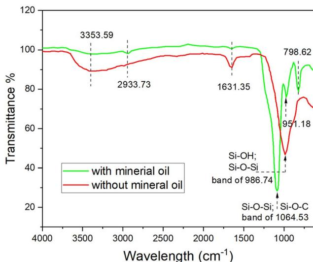
Fig. 4 The ATR-FTIR spectra of SiO<sub>2</sub> synthesized with the presence of mineral oil and without mineral oil.
