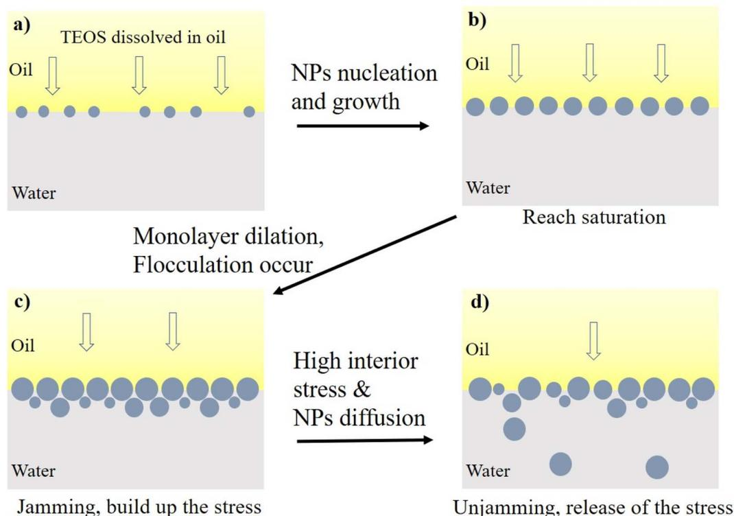
Fig. 11 The states of oil–water interface saturated with *in situ* produced silica NPs. (a) Unsaturated interface with large interparticle distances; (b) the interface saturated with monolayer particles; (c) particle jamming to build up the stress; (d) particle unjamming to release the stress.
