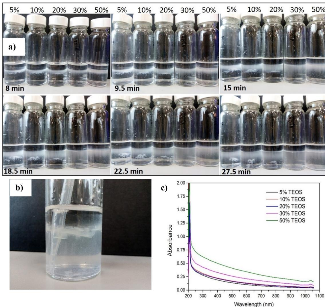
Fig. 7 The reaction rate for samples with 10%  $\text{NH}_4\text{OH}$ . (a) Samples starting from 8 min to 27.5 min; (b) the mashed interface where the silica NPs formed, for sample with 5% TEOS; (c) the UV-vis adsorption of aqueous phase at 27.5 min.
