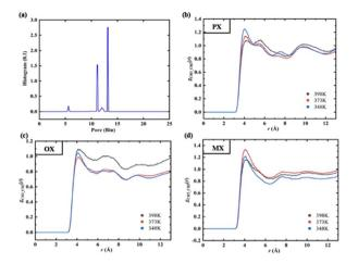
Fig. 5 (a) Histogram of the pore size distribution (PSD). (b–d) RDF between  $-CH_3$  group of xylenes at different temperatures.
