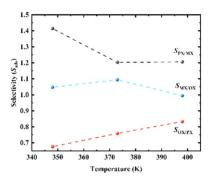
Fig. 7 Selectivity values ( $S_{ads}$ ) for separation of binary mixtures of xylenes on Cu-HKUST-1 at 1000 Pa.
