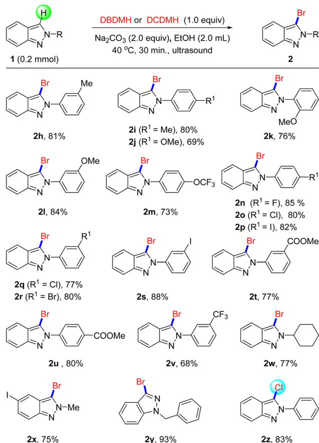
Scheme 2 The Halogenation of Indazoles. <sup>a</sup>Reaction conditions: **1** (0.2 mmol), DBDMH (0.2 mmol), Na<sub>2</sub>CO<sub>3</sub> (0.4 mmol), 40 °C, EtOH (2.0 mL), ultrasonic 30 min <sup>b</sup>DCDMH (0.2 mmol).
