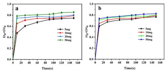
Fig. 5 The effect of the amount of Co/Cu-MOFs (a) and PMS (b) on degradation.
