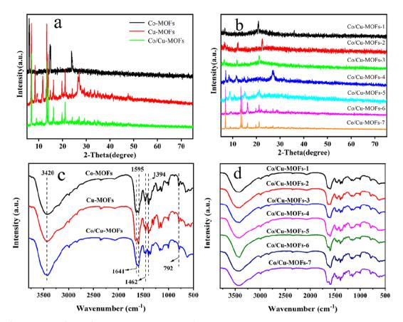
Fig. 1 (a and b) XRD patterns, (c and d) FT-IR spectra of different MOFs
