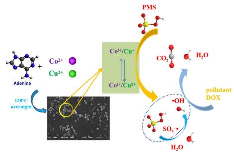
Fig. 7 Schematic illustration of the reaction mechanisms in the Co/Cu-MOFs/PMS system
