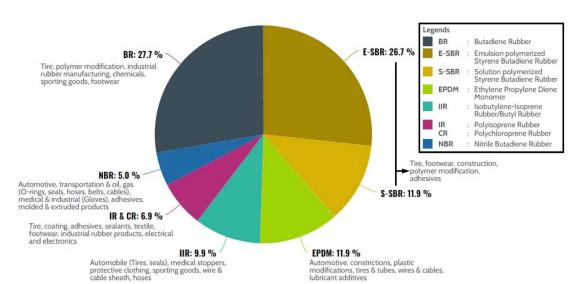
Fig. 4 Demand for synthetic rubber in 2020 according to rubber types, and their respective applications.<sup>49–57</sup>
