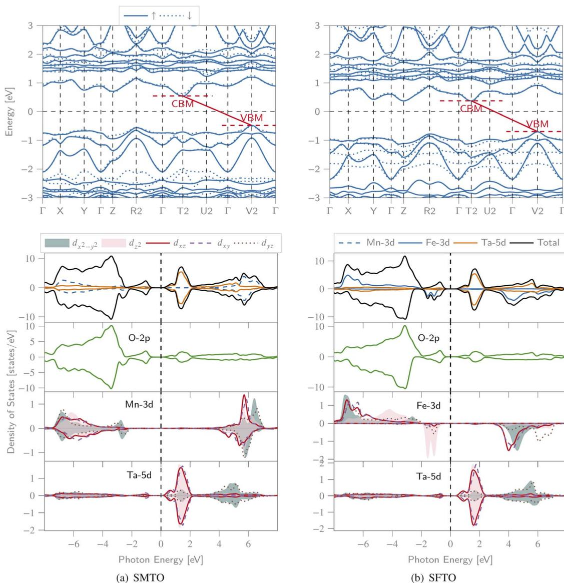
Fig. 3 The spin polarized band structure (upper), total DOS and PDOS (lower) of the (a) SMTO and (b) SFTO compounds computed employing GGA +  $U$ ,  $U_{41}$  approximation ( $U_{\text{Mn,Fe}} = 4.0$  eV and  $U_{\text{Ta}} = 1.0$  eV). The Fermi level is set as zero. CBM: conduction band minimum, VBM: valence band maximum. Both structures exhibit a semiconducting nature with band gaps slightly larger than 1.0 eV in both spin states, see Table 3 for details.
