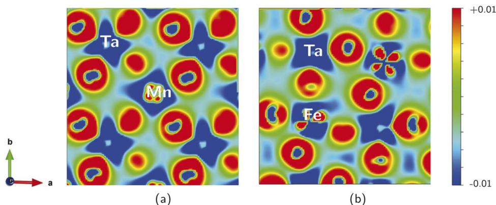
Fig. 4 Charge density difference plots ( $e/\text{\AA}^3$ ), describing the charge distribution difference between the optimized and initial structures, in (001) plane for (a) SMTO and (b) SFTO compounds. Positive (negative) values show the charge accumulated (depleted) regions. The charge sharing between the Mn/Fe-O and Ta-O atoms in  $Mn/FeO_6$  and  $TO_6$  octahedra show the covalent nature, and p-d hybridization.
