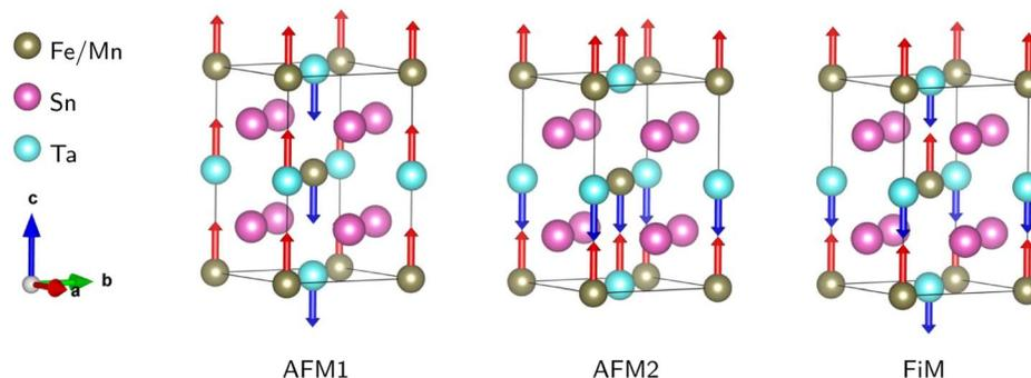
Fig. 2 Different magnetic configurations of the conventional cell for the  $\text{Sn}_2\text{Mn/FeTaO}_6$  DPs; AFM1, 2: antiferromagnetic; FiM: ferrimagnetic. Total energy calculations show that AFM2 and FM orderings are the magnetic ground states for SMTO and SFTO, respectively, resulting from a superexchange interaction between Mn/Fe-3d half-field and Ta-5d empty orbitals following the Goodenough–Kanamori rule.
