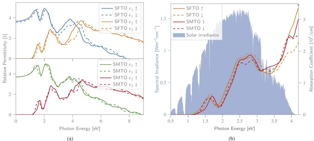
Fig. 5 (a) Spin-dependent real  $\epsilon_1$  and imaginary  $\epsilon_2$  parts of dielectric function, (b) absorption spectra, as a function of photon energy calculated for SMTO and SFTO systems using GGA +  $U$ , together with the AM1.5g solar irradiance spectrum.<sup>48</sup> All spin states exhibit a non-vanishing absorption behaviour within a wide, PV-relevant spectral range between 1.3 and 4.2 eV.
