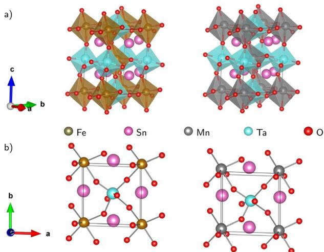
Fig. 1 Schematic representation of the  $Sn_2MnTaO_6$  and  $Sn_2FeTaO_6$  double perovskites conventional unit cell in (a) polyhedral form and (b) top view of the atomic form. The deviation of B–O–B' bond angles from  $180^\circ$  indicating significant buckling of the octahedral connection. The Jahn–Teller effect is responsible for the  $BO_6$  and  $B'O_6$  octahedra distortion resulting in B/B'–O bond length changes (see  $\langle \omega \rangle$  and  $\Delta d$  in Table 2).
