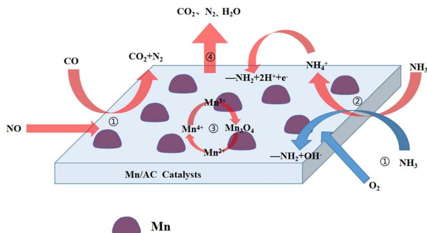
Fig. 8 Mechanism of low-temperature CO + NH<sub>3</sub> coupling denitration diagram of Mn/AC catalysts.
