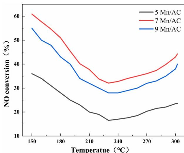
Fig. 2 NO conversion rate of the Mn/AC catalysts.
