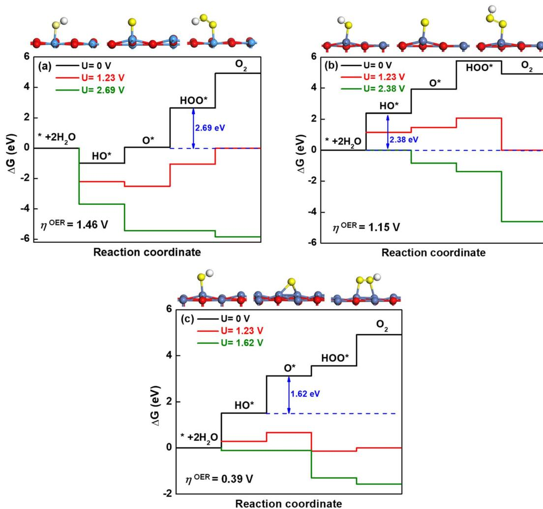
Fig. 7 Free-energy diagram at pH = 0 and  $T = 298$  K for the four steps of the OER at different applied potentials. The relaxed structures of intermediates are attached, in which the light blue, red, dark blue, yellow, and white balls represent the Ta, O in the surface, Ni, O in water, and H atoms, respectively.
