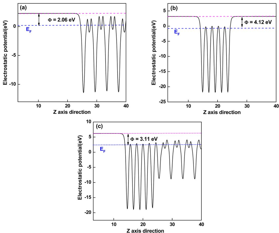
Fig. 5 Calculated electrostatic potentials of (a) KTaO<sub>3</sub>(001), (b) NiO(001), and (c) NiO(001)/KTaO<sub>3</sub>(001) heterostructure. The magenta and blue dashed lines indicate the vacuum energy level and Fermi level, respectively.
