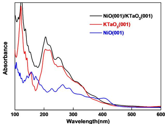
Fig. 6 Computed optical absorption curves of NiO(001)/KTaO<sub>3</sub>(001), KTaO<sub>3</sub>(001) and NiO(001) slab models.
