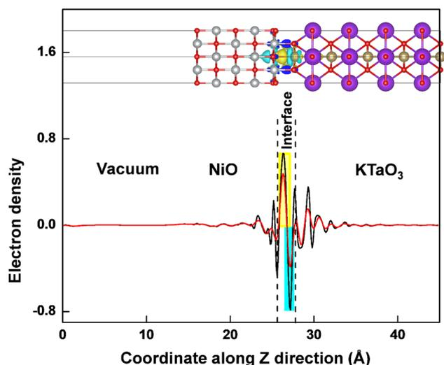
Fig. 4 The three-dimensional charge density differences and the corresponding planar average differences (black line) and integral charge transfer (red line) for NiO(001)/KTaO<sub>3</sub>(001) interface. The yellow and cyan regions indicate electron accumulation and depletion, respectively. The isosurface value is 0.002 e Å<sup>-3</sup>.
