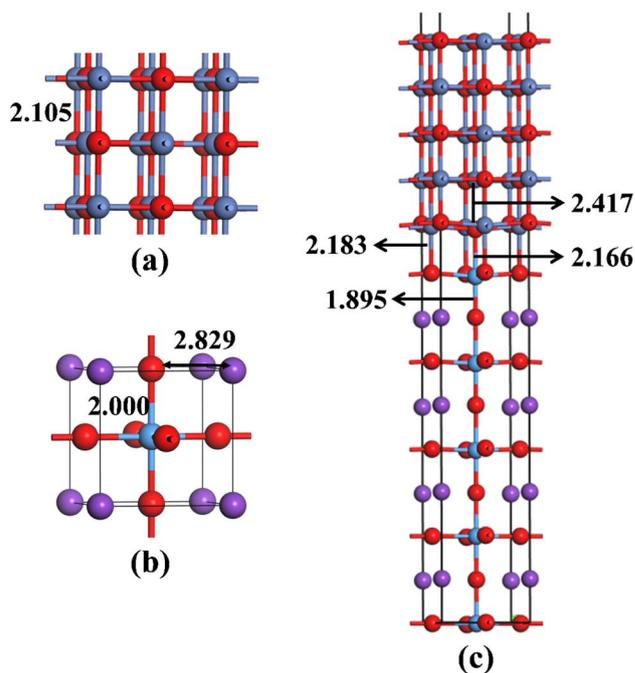
Fig. 1 Optimized structures of (a) bulk NiO, (b) bulk  $\text{KTaO}_3$ , and (c) NiO(001)/ $\text{KTaO}_3(001)$  interface with key bond lengths. The red, blue, purple and azure balls represent O, Ni, K and Ta atoms, respectively.
