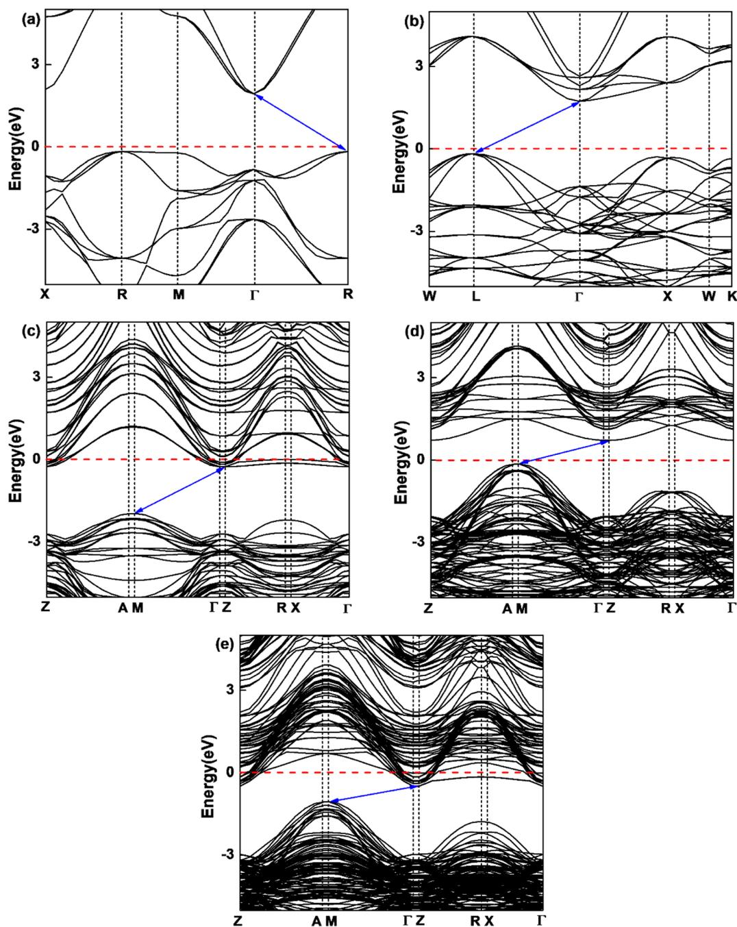
Fig. 2 Calculated band structures of (a) bulk KTaO<sub>3</sub> and (b) bulk NiO, (c) KTaO<sub>3</sub>(001), (d) NiO(001), and (e) NiO(001)/KTaO<sub>3</sub>(001). The Fermi level is set to be zero as a horizontal dashed red line.
