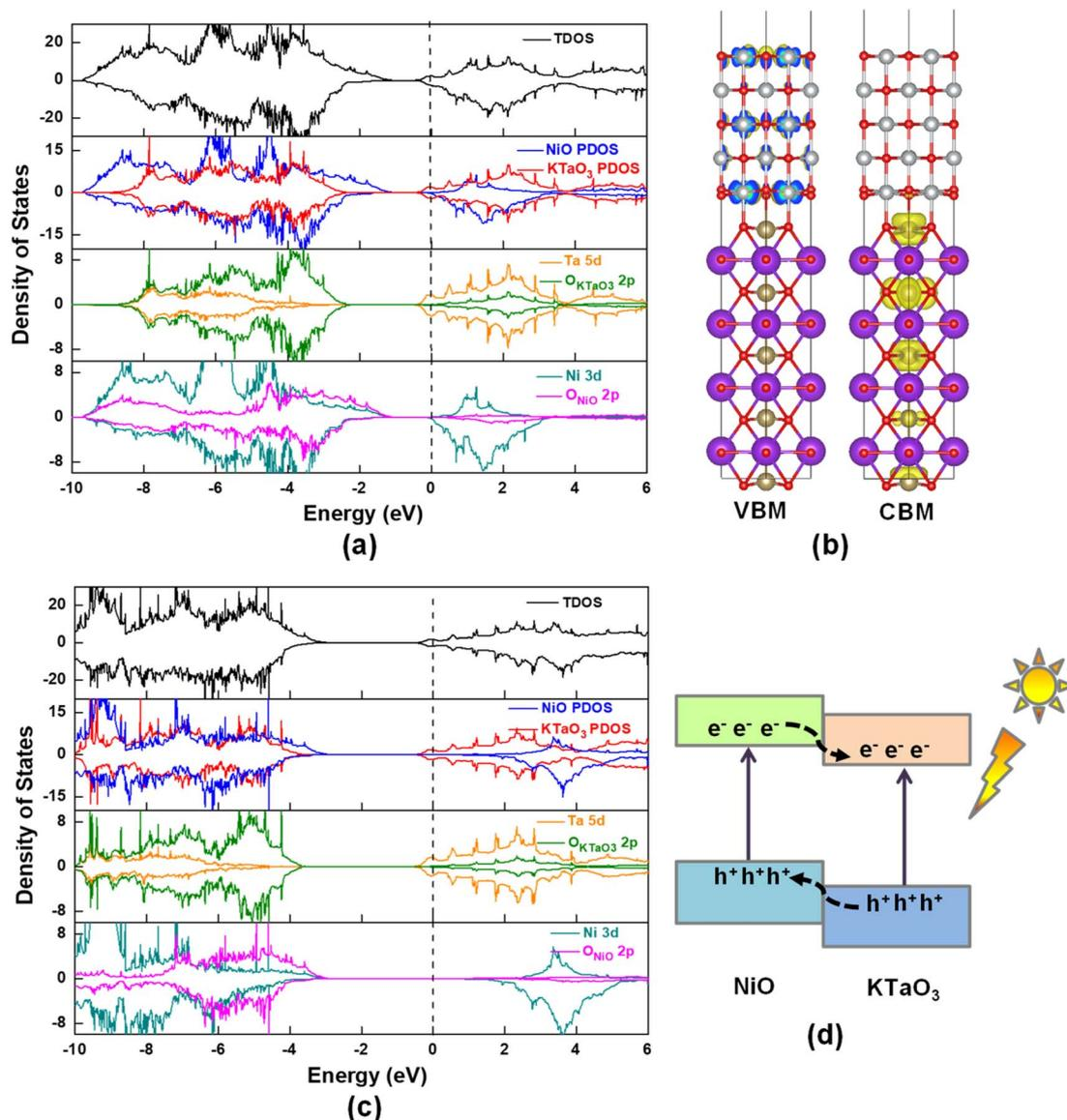
Fig. 3 (a) Calculated TDOS and PDOS of NiO(001)/KTAO<sub>3</sub>(001) by using PBE+U method, (b) the charge density distributions of VBM and CBM obtained by VESTA, (c) calculated TDOS and PDOS by using HSE06 method, (d) the band alignment of two components in NiO(001)/KTAO<sub>3</sub>(001).
