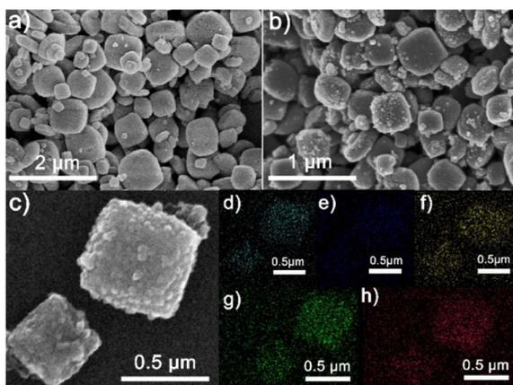
Fig. 2 SEM images of NH<sub>2</sub>-MIL-125(Ti) (a), NTiPC (b) and S/NTiPC (c), respectively. The elemental mapping of carbon (d), nitrogen (e), oxygen (f), titanium (g) and sulfur (h) of S/NTiPC.
