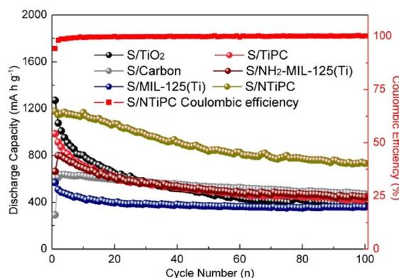
Fig. 6 The discharge capacity of S/MIL-125(Ti), S/TiPC, S/NH<sub>2</sub>-MIL-125(Ti) and S/NTiPC cathodes and the coulombic efficiency of S/NTiPC cathode at 0.5C during 100 cycles.
