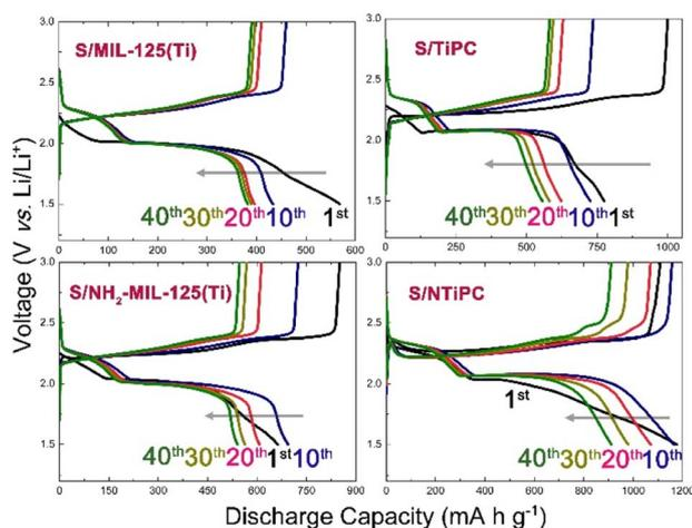
Fig. 5 Discharge/charge curves of the S/MIL-125(Ti), S/TiPC, S/NH<sub>2</sub>-MIL-125(Ti) and S/NTiPC cathodes and the coulombic efficiency of S/NTiPC cathodes at different cycles at 0.5C.
