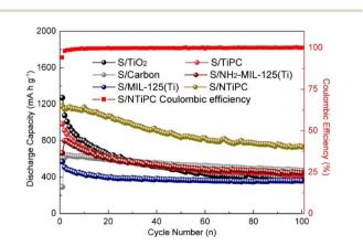
Fig. 6 The discharge capacity of S/MIL-125(Ti), S/TiPC, S/NH $_2$ -MIL-125(Ti) and S/NTiPC cathodes and the coulombic efficiency of S/NTiPC cathode at 0.5C during 100 cycles.
