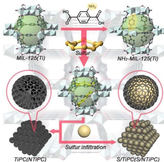
Fig. 1 Ball and stick representation of the octahedral cage of MIL-125 and NH<sub>2</sub>-MIL-125, the large light green sphere represents the effective accessible volume of the cage. The illustration of MIL-125(Ti) and NH<sub>2</sub>-MIL-125(Ti) after carbonization under an N<sub>2</sub> atmosphere, and the S/MIL-125(Ti) and S/NH<sub>2</sub>-MIL-125(Ti) composites preparation.
