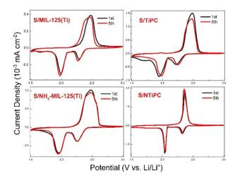
Fig. 4 CV curves of in a range of S/MIL-125(Ti), S/TiPC, S/NH<sub>2</sub>-MIL-125(Ti) and S/NTiPC cathodes 1.5-3 V with a scanning rate of 0.1 mV  $s^{-1}$
