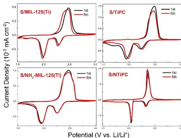
Fig. 4 CV curves of in a range of S/MIL-125(Ti), S/TiPC, S/NH<sub>2</sub>-MIL-125(Ti) and S/NTiPC cathodes 1.5–3 V with a scanning rate of 0.1 mV s<sup>-1</sup>.
