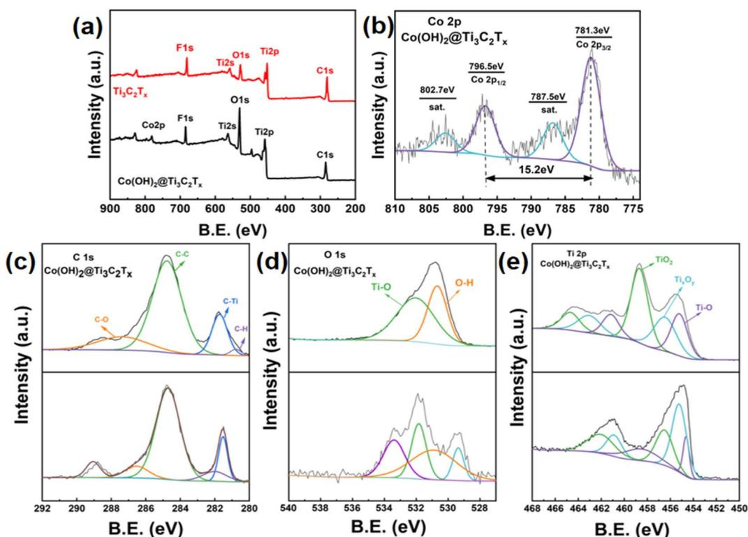
Fig. 4 (a) Full survey XPS spectrum of  $\text{Co(OH)}_2/\text{Ti}_3\text{C}_2\text{T}_x$ . High-resolution XPS spectra for (b) Co 2p of  $\text{Co(OH)}_2/\text{Ti}_3\text{C}_2\text{T}_x$  hybrids. High-resolution XPS spectra for (c) C 1s, (d) O 1s and (e) Ti 2p of  $\text{Co(OH)}_2/\text{Ti}_3\text{C}_2\text{T}_x$  hybrids and  $\text{Ti}_3\text{C}_2\text{T}_x$  MXene.
