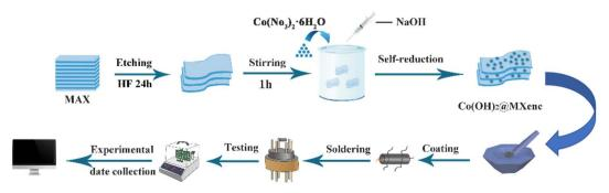
Fig. 1 Schematic illustration of the experimental procedure.
