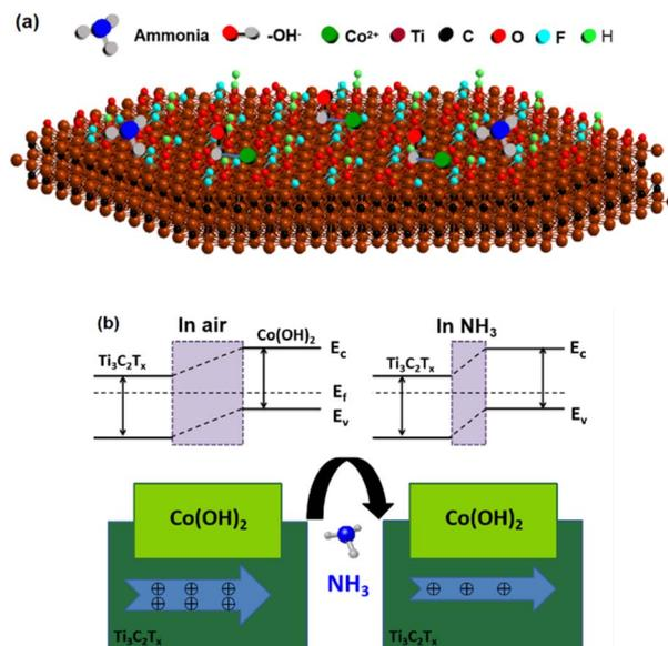
Fig. 8 (a) Schematic of the reaction between  $\text{NH}_3$  and  $\text{Co}(\text{OH})_2/\text{Ti}_3\text{C}_2\text{T}_x$  composite. (b) Energy band structure diagram and conductivity pathway of the  $\text{Co}(\text{OH})_2/\text{Ti}_3\text{C}_2\text{T}_x$  hybrid sensor before and after  $\text{NH}_3$  molecules absorption.
