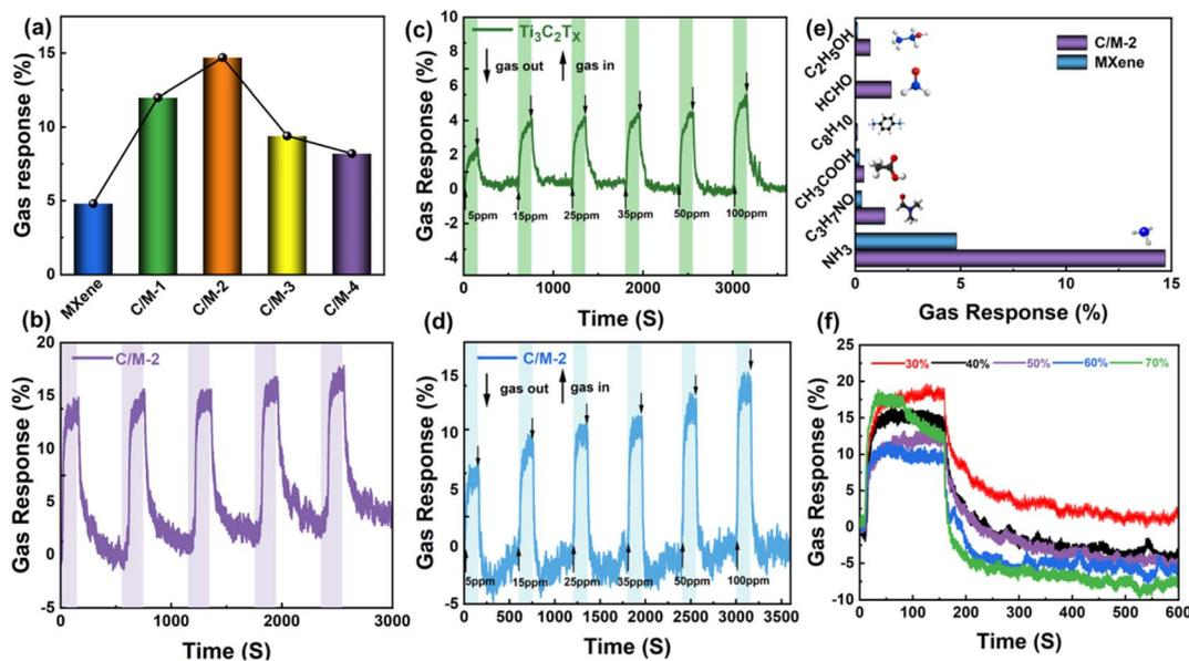
Fig. 6 (a) Response of all samples to 100 ppm  $\text{NH}_3$ . (b) Repeatability of C/M-2 sensor toward 100 ppm  $\text{NH}_3$  at room temperature. (c)  $\text{Ti}_3\text{C}_2\text{T}_x$  and (d) C/M-2 sensor to 5–100 ppm  $\text{NH}_3$ . (e) Selectivity of the C/M-2 and  $\text{Ti}_3\text{C}_2\text{T}_x$  sensor to various gases at room temperature. (f) Dynamic response–recovery curves of the C/M-2 sensor at 30–70% RH towards 100 ppm  $\text{NH}_3$ .
