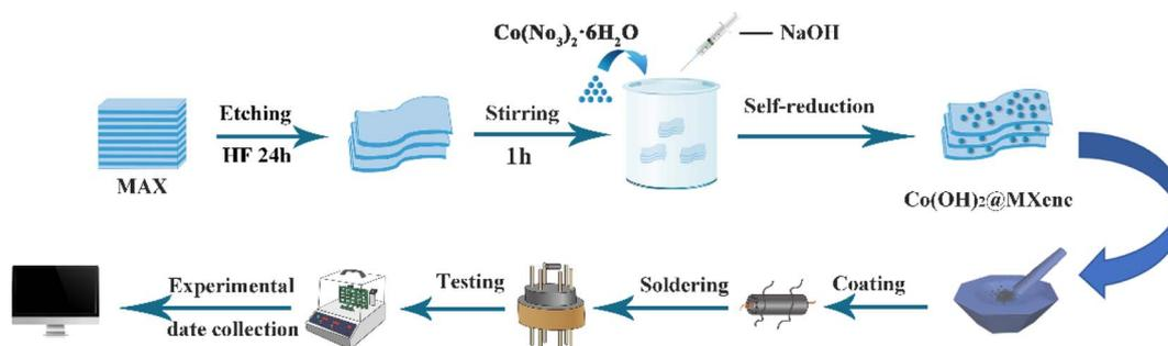
Fig. 1 Schematic illustration of the experimental procedure.
