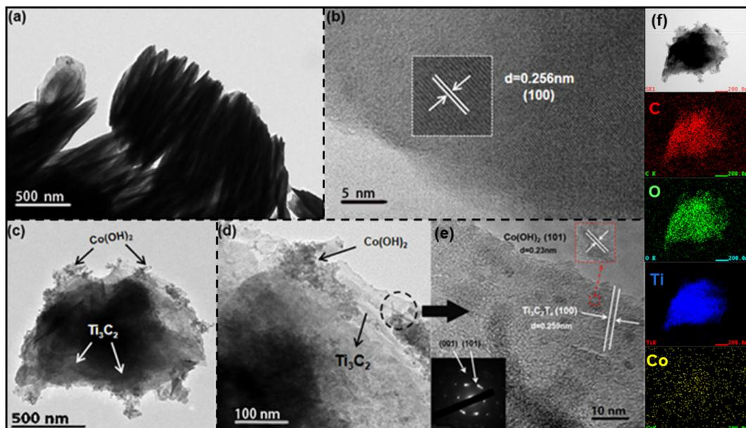
Fig. 3 (a) TEM and (b) HRTEM images of  $\text{Ti}_3\text{C}_2\text{T}_x$  MXene. (c and d) TEM and (e) HRTEM images of  $\text{Co(OH)}_2/\text{Ti}_3\text{C}_2\text{T}_x$  hybrids (f) HADDF image of  $\text{Co(OH)}_2/\text{Ti}_3\text{C}_2\text{T}_x$  hybrids and corresponding elemental mapping of C, Ti, Co, and O.
