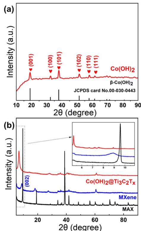
Fig. 2 XRD patterns of (a) Co(OH)<sub>2</sub> and (b) Ti<sub>3</sub>C<sub>2</sub>T<sub>x</sub> MXene and MAX and the Co(OH)<sub>2</sub>/Ti<sub>3</sub>C<sub>2</sub>T<sub>x</sub> hybrids (2.13 wt%).
