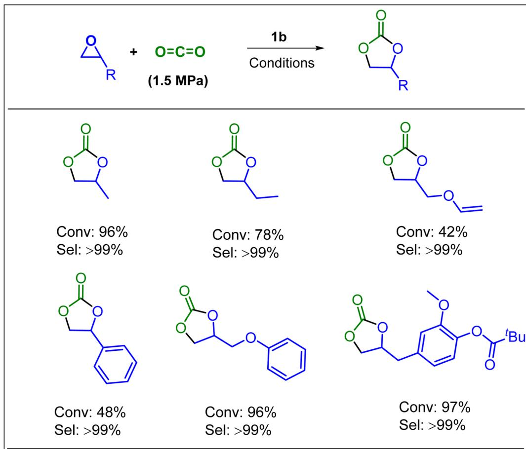
**Scheme 1** Synthesis of cyclic carbonates from various epoxides and CO<sub>2</sub> using organocatalysts **1b**. The reaction was performed epoxide (9.9 mmol; 1.5 MPa CO<sub>2</sub>; catalyst/epoxides = 1/1000) in a 15 mL autoclave using toluene/CH<sub>2</sub>Cl<sub>2</sub> (0.8 mL) at 80 °C for 18 h.
