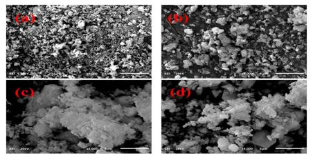
Fig. 5 FESEM images of (a) CaO, (b) St-CaO, (c) Al (2%)/St-CaO and (d) Al (4%)/St-CaO.
