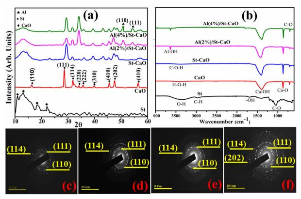
Fig. 3 (a) XRD spectra, (b) FTIR analysis of prepared samples and (c-f) SAED pattern of CaO, St/CaO, and Al (2 and 4%)/St-CaO.
