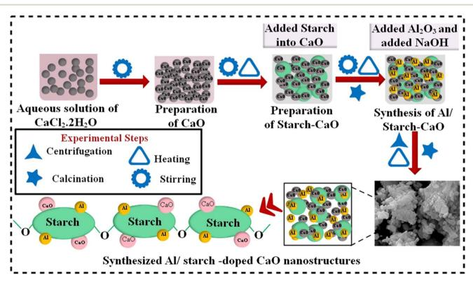
Fig. 1 Schematic diagram of the synthesis of Al/St-doped CaO NPs.
