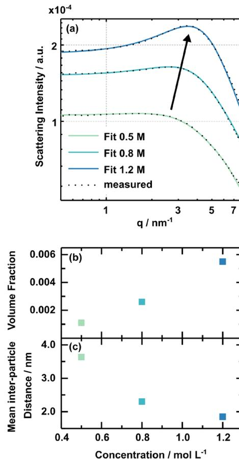
Fig. 4 SAXS data on the 3CatPbBr<sub>3</sub> solution concentration series. The scattering intensity is illustrated in (a) for 0.5 M, 0.8 M, and 1.2 M concentrated solutions with black dots representing the raw data and solid lines the fit. (b) Demonstrates the concentration dependency of the structural factor, namely the volume fraction and (c) the mean inter-particle distance. *R*-values for the fits are 0.0114 (0.5 M), 0.0033 (0.8 M) and 0.0038 (1.2 M).
