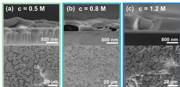
Fig. 1 SEM images of the final 3CatPbBr<sub>3</sub> films prepared from the solution concentration series, (a) 0.5 M, (b) 0.8 M, (c) 1.2 M. The top row presents the cross-section, while the bottom row presents the top view images. All three concentrations result in rough and incomplete films regarding coverage and morphology.
