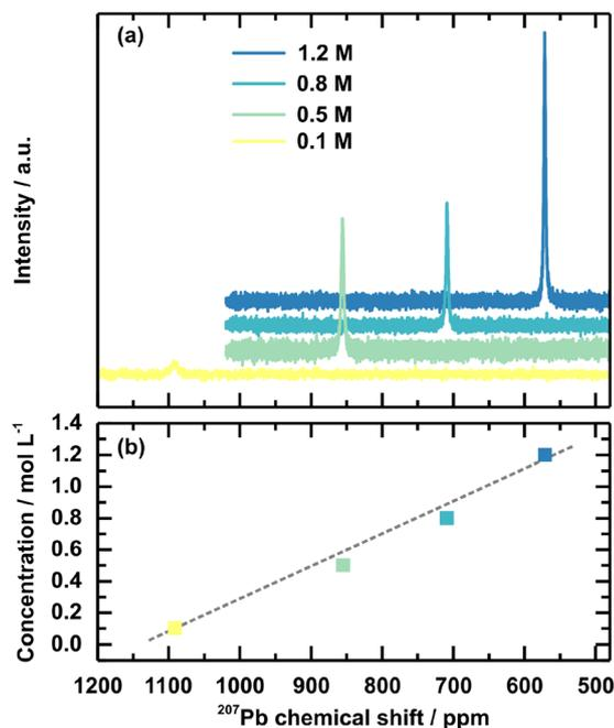
Fig. 5  $^{207}\text{Pb}$  NMR spectra (a) of the 3CatPbBr<sub>3</sub> solution concentration series and an additional diluted 0.1 M solution. (b) Visualises the dependency of the  $^{207}\text{Pb}$  chemical shift on the concentration. The grey dashed line gives a guide for the eye of the linear dependency.
