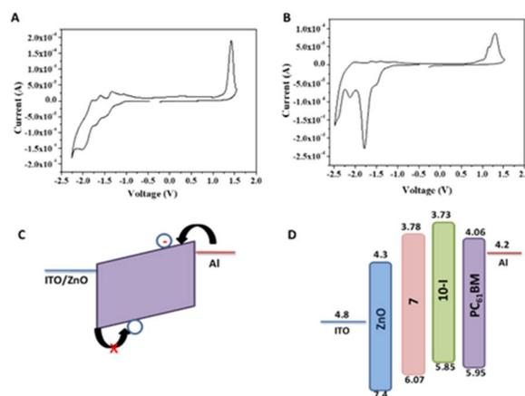
Fig. 9 Cyclic voltammetry curves of (A) 7 and (B) **10-I** (v/s Fc/Fc<sup>+</sup>) with 0.1 M *n*-Bu<sub>4</sub>NPF<sub>6</sub> as a supporting electrolyte and scan rate 100 mV s<sup>-1</sup>. (C) Schematic representation of fabricated electron-only device and (D) energy level diagram with HOMO and LUMO values.
