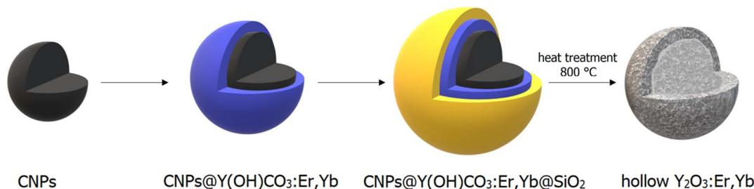
**Scheme 1** Schematic overview of the preparation of Y<sub>2</sub>O<sub>3</sub>:Er,Yb hollow spheres, starting from carbon nanoparticles (CNPs). A shell of Y(OH)CO<sub>3</sub>:Er,Yb was first grown around the CNPs, which were then coated with a layer of SiO<sub>2</sub> and subsequently heat-treated to obtain Y<sub>2</sub>O<sub>3</sub>:Er,Yb hollow spheres.
