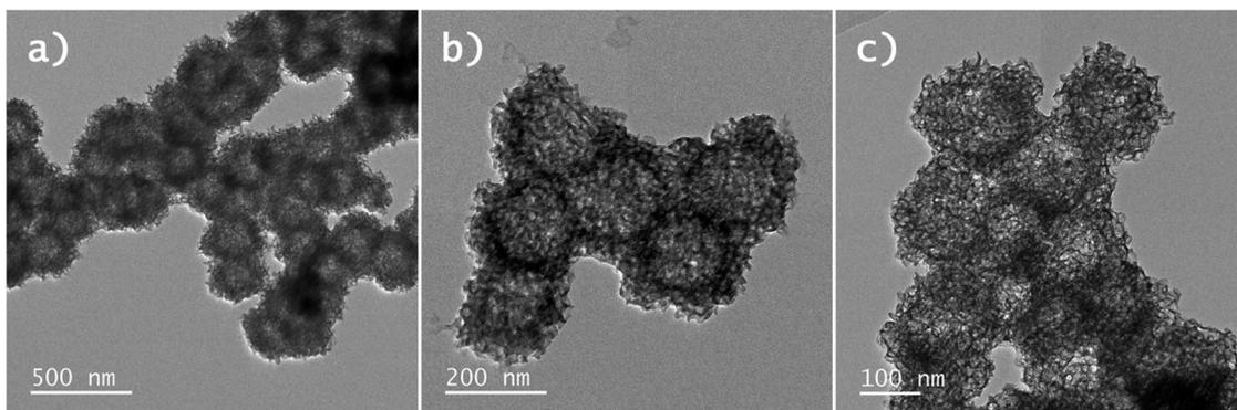
Fig. 4 BF-STEM images of (a) and (b)  $\text{Y}_2\text{O}_2\text{SO}_4\text{:Er,Yb}$  precursor and (c)  $\text{Y}_2\text{O}_2\text{SO}_4\text{:Er,Yb}$  hollow spheres obtained after heat-treatment in air.
