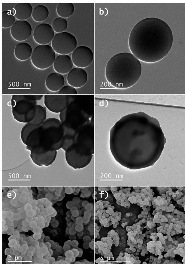
**Fig. 1** BF-STEM images of (a) and (b) CNPs obtained in the hydrothermal synthesis and (c) and (d) CNPs@Y(OH)CO<sub>3</sub>:Er,Yb spheres and (e) and (f) SEM images of CNPs@Y(OH)CO<sub>3</sub>:Er,Yb spheres.
