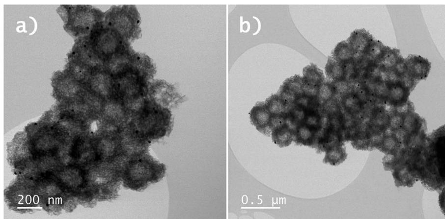
Fig. 9 (a) and (b) BF-STEM images  $\text{Y}_2\text{O}_2\text{SO}_4:\text{Er,Yb}@Au\text{NPs}$  precursors hollow spheres. The AuNPs can be observed as small black dots on the surface of the  $\text{Y}_2\text{O}_2\text{SO}_4:\text{Er,Yb}@Au\text{NPs}$  hollow spheres.
