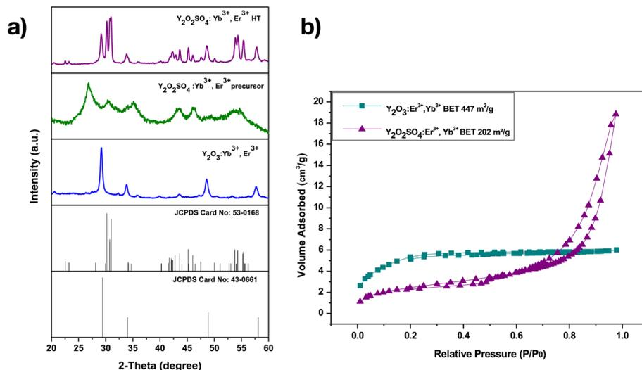
Fig. 6 (a) Powder XRD patterns of  $\text{Y}_2\text{O}_3:\text{Er},\text{Yb}$  and  $\text{Y}_2\text{O}_2\text{SO}_4:\text{Er},\text{Yb}$  (before "precursor" and after heat treatment "HT" at 850 °C for 3 h), (b)  $\text{N}_2$  sorption isotherms for  $\text{Y}_2\text{O}_3:\text{Er},\text{Yb}$  and  $\text{Y}_2\text{O}_2\text{SO}_4:\text{Er},\text{Yb}$  precursor.
