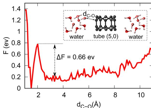
**Fig. 3** Energy profile and activation barrier of H<sub>2</sub>O splitting on the surface of tube (5,0) obtained from metadynamics simulations at  $T = 298.15 \text{ K}$ .
