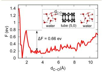
Fig. 3 Energy profile and activation barrier of  $\rm H_2O$  splitting on the surface of tube (5,0) obtained from metadynamics simulations at  $T=298.15~\rm K$ .
