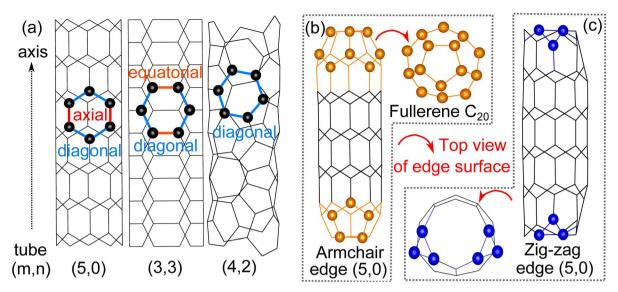
Fig. 1 (a) Stick model of 4 Å SWCNTs: tube (5,0), (3,3) and (4,2) with the carbon atoms of one hexatomic ring represented by balls for clarity, (b) ball and stick model of tube (5,0) with armchair edges that fold into half fullerene  $C_{20}$  and (c) ball and stick model of tube (5,0) with zig-zag edges that have an irregular edge surface.
