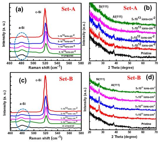
Fig. 4 (a) Raman spectra (b) XRD pattern of set-A irradiated by 100 MeV Ni ions at 100 °C with different fluence of  $1 \times 10^{12}$  ions per cm²,  $5 \times 10^{12}$  ions per cm²,  $1 \times 10^{13}$  ions per cm², and  $5 \times 10^{13}$  ions per cm². And (c) Raman spectra (d) XRD of set-B irradiated at 100 °C with different fluences at 100 °C with different fluence of  $1 \times 10^{12}$  ions per cm²,  $5 \times 10^{12}$
