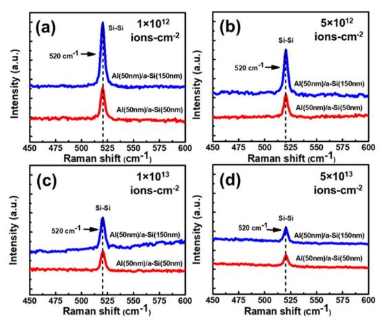
Fig. 7 Raman spectra of set-A and set-B samples irradiated at 100 °C with different fluences of (a)  $1 \times 10^{12}$  ions per cm<sup>2</sup>, (b)  $5 \times 10^{12}$  ions per  $\text{cm}^2$ , (c)  $1 \times 10^{13}$  ions per  $\text{cm}^2$ , and (d)  $5 \times 10^{13}$  ions per  $\text{cm}^2$ . (All figures are plotted in same y-scale range for comparison). [Reproduced/adapted from Maity et al., 157 RSC Adv., 2020, 10, 4414, with permission from The Royal Society of Chemistry.]
