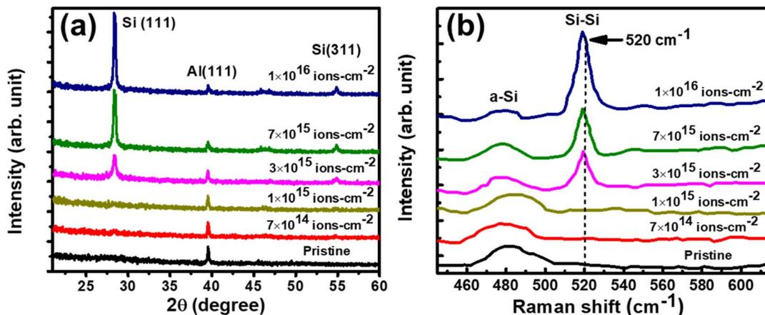
Fig. 10 (a) XRD pattern (b) Raman spectra of pristine sample and the samples irradiated with different ion fluence of  $7 \times 10^{14}$  ions per  $\text{cm}^2$ ,  $1 \times 10^{15}$  ions per  $\text{cm}^2$ ,  $3 \times 10^{15}$  ions per  $\text{cm}^2$ ,  $7 \times 10^{15}$ , and  $1 \times 10^{16}$  ions per  $\text{cm}^2$ . [Reproduced/adapted from Maity *et al.*,<sup>161</sup> *J. Appl. Phys.*, 2022, 132, 095303, with the permission from AIP Publishing.]
