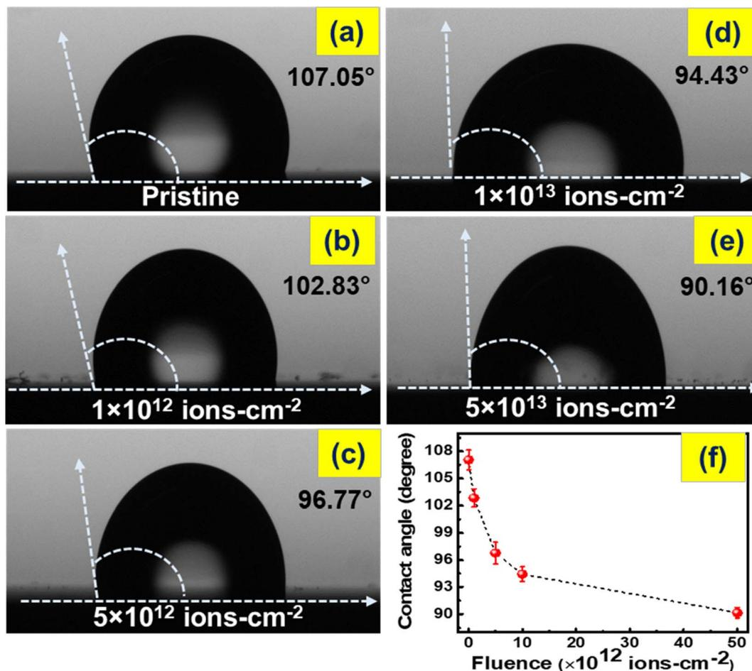
Fig. 14 Contact angles (CA) of (a) pristine film, and absorber films developed at different fluences of (b)  $1 \times 10^{12}$  ions per  $\text{cm}^2$ , (c)  $5 \times 10^{12}$  ions per  $\text{cm}^2$ , (d)  $1 \times 10^{13}$  ions per  $\text{cm}^2$ , and (e)  $5 \times 10^{13}$  ions per  $\text{cm}^2$ . (f) Variation of CA with ion fluence. [Reproduced/adapted from Maity *et al.*,<sup>159</sup> *J. Appl. Phys.*, 2021, 129, 045301, with the permission from AIP Publishing.]
