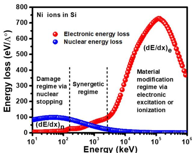
Fig. 2 Variation of energy loss of Ni ions in Si using SRIM-2008 simulation code.
