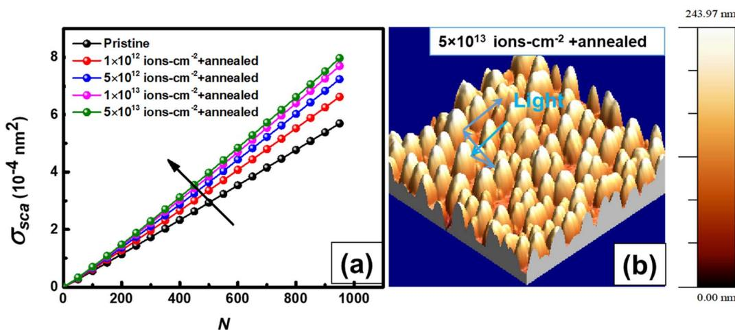
Fig. 16 (a) Scattering cross section ( $\sigma_{sca}$ ) as a function of number of constituent grain ( $N$ ) on film surface (b) three-dimensional AFM image of post-annealed (at 300 °C) sample irradiated at fluence of 5 × 10<sup>13</sup> ions per cm<sup>2</sup> to demonstrate the schematic of multiple scattering of light. [Reproduced/adapted from Maity *et al.*,<sup>162</sup> *CrystEngComm.*, 2020, 22, 666, with permission from The Royal Society of Chemistry.]
