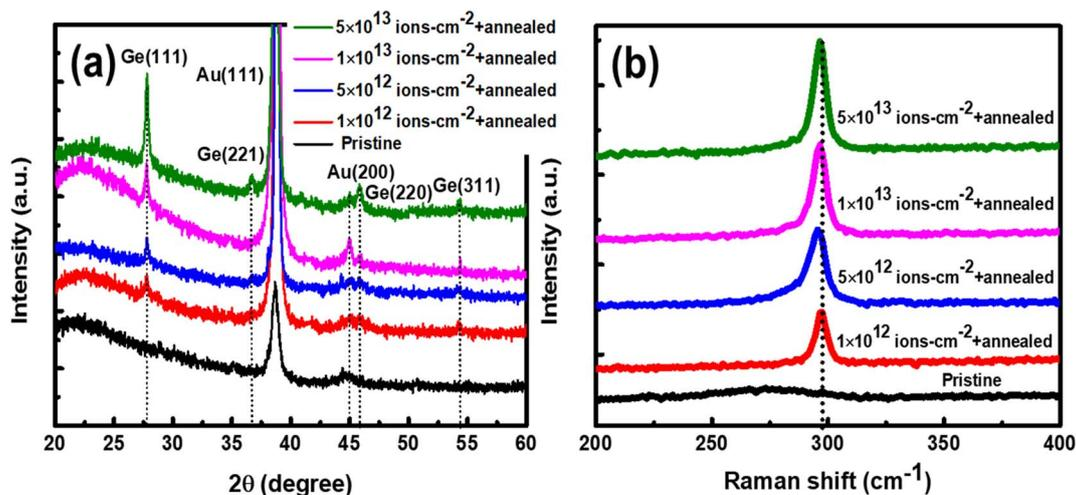
Fig. 12 (a) XRD pattern and (b) Raman spectra of pristine sample and samples post-annealed (after ion irradiation at different fluences) at 300 °C. The XRD and Raman results clearly show the crystallization of Ge due to thermal annealing treatment after ion irradiation. [Reproduced/adapted from Maity *et al.*,<sup>162</sup> *CrystEngComm*, 2020, 22, 666, with permission from The Royal Society of Chemistry.]
