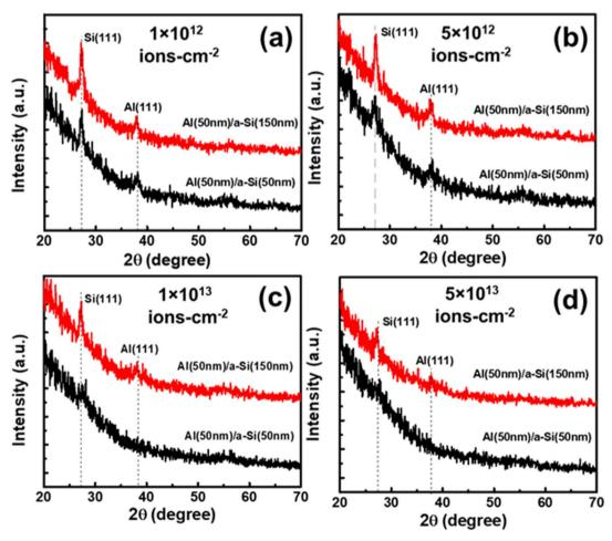
Fig. 8 GIXRD pattern of set-A and set-B samples irradiated at 100 °C with different fluences of (a)  $1 \times 10^{12}$  ions per cm<sup>2</sup>, (b)  $5 \times 10^{12}$  ions per cm<sup>2</sup>, (c)  $1 \times 10^{13}$  ions per cm<sup>2</sup>, and (d)  $5 \times 10^{13}$  ions per cm<sup>2</sup>. (All figures are plotted in same y-scale range for comparison). [Reproduced/adapted from Maity et al., 157 RSC Adv., 2020, 10, 4, 414, with permission from The Royal Society of Chemistry.]
