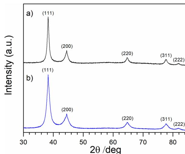
Fig. 7 XRD patterns of thin layers prepared by casting on a Si(510) zero diffraction substrate from AuNPs-2 (a) and AuNPs-5 (b) colloids.
