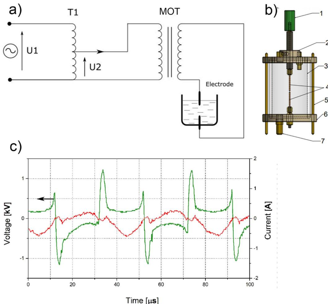
Fig. 1 (a) Diagram of a submerged continuous arc discharge reactor. (1) Adjusting screw, (2) top cover with gas dosing valve and first electrode clamp. (3) Borosilicate glass tube filled with water. (4) Wire gold electrodes (5) bottom cover with holder for the second electrode. (b) Scheme of power supply. (c) Current–voltage characteristic during AC arc discharge.
