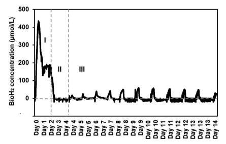
Fig. 3 The sequential bioH<sub>2</sub> production in the SFBR during phase I (exponential), II (lag), and III (steady-state).
