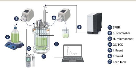
Fig. 1 A schematic of the studied SFBR unit setup.
