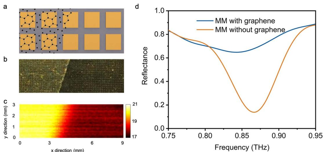
**Fig. 2** THz imaging of monolayer graphene-coated THz metamaterial device. (a) Schematic of THz imaging area, including THz metamaterial with/without graphene. (b) Photograph of THz metamaterial device, the area is according to (a). (c) THz imaging of metamaterial device with/without graphene at 0.85 THz. (d) THz reflection spectrum of metamaterial device with/without graphene.
