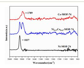
Fig. 11 In situ DRIFTS spectra of as-prepared Ni-MOF-74, Co-MOF-74 and Ni<sub>0.37</sub>Co<sub>0.63</sub>-MOF-74.
