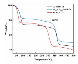
Fig. 2 TG curve of Co-MOF-74, Ni-MOF-74 and Ni<sub>0.37</sub>Co<sub>0.63</sub>-MOF-74.
