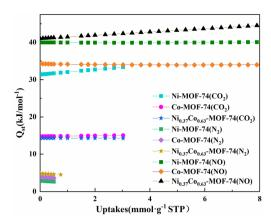
Fig. 10  $CO_2$ ,  $N_2$  and NO adsorption enthalpy of Co-MOF-74, Ni-MOF-74 and Ni<sub>0.37</sub>Co<sub>0.63</sub>-MOF-74.
