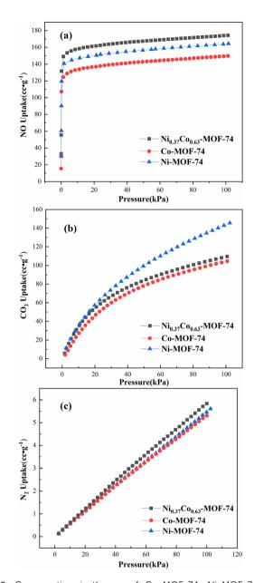
Fig. 5 Gas sorption isotherms of Co-MOF-74, Ni-MOF-74 and Ni $_{0.37}$ Co $_{0.63}$ -MOF-74 for NO (a), CO $_2$  (b) and N $_2$  (c) at 298 K.
