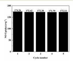
Fig. 7 The adsorption capacity of  $Ni_{0.37}Co_{0.63}$ -MOF-74 for NO at different regeneration times at 100 kPa.
