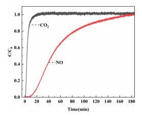
Fig. 9 The breakthrough curve of Ni<sub>0.37</sub>Co<sub>0.63</sub>-MOF-74.
