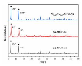
Fig. 1 PXRD spectra of Co-MOF-74, Ni-MOF-74 and  $Ni_{0.37}Co_{0.63}$ -MOF-74.
