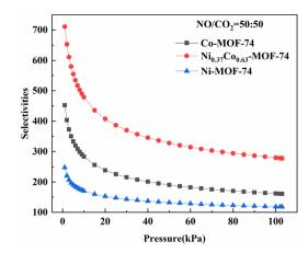
Fig. 6 Adsorption selectivity of Co-MOF-74, Ni-MOF-74 and Ni<sub>0.37</sub>Co<sub>0.63</sub>-MOF-74 for NO/CO<sub>2</sub> predicted by IAST model (298 K).
