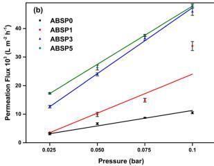
Fig. 9 Performance evaluation of ENMs (a) permeation flux at a fixed pressure (0.025 bar), and (b) permeation flux as a function of pressures.
