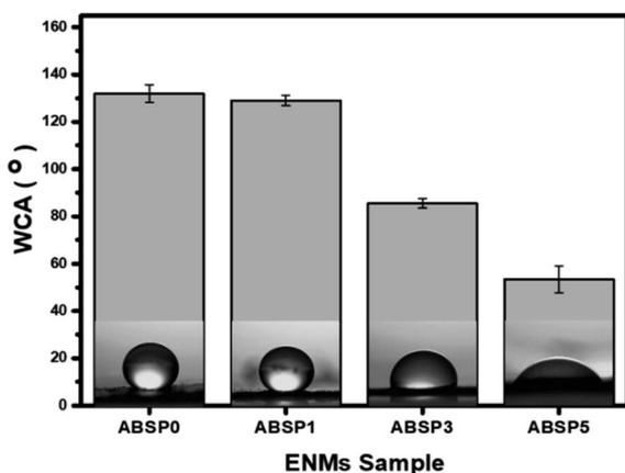
Fig. 8 Water contact angle measurement of ENMs.
