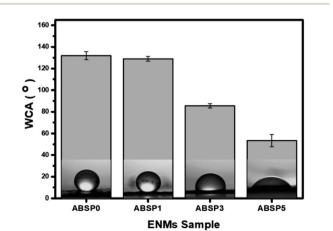
Fig. 8 Water contact angle measurement of ENMs.
