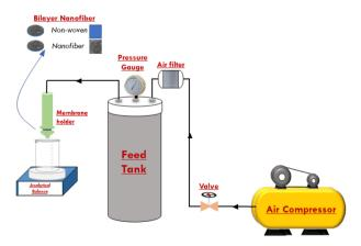
Fig. 1 Schematic of ENMs performance evaluation system.
