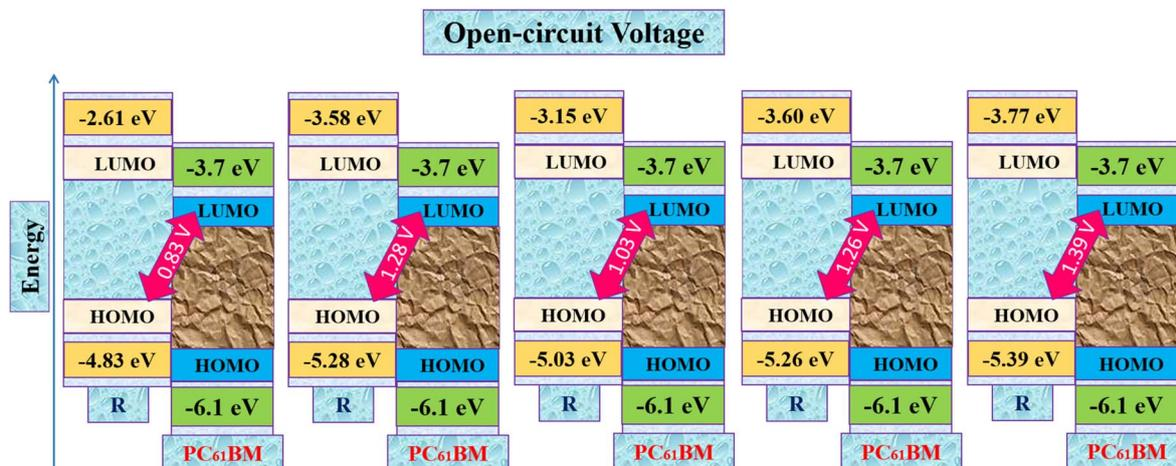
Fig. 12  $V_{OC}$  of proposed compounds, as well as the reference molecule, calculated using PC<sub>61</sub>BM as the acceptor.
