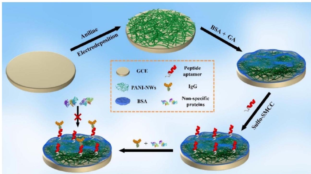
Fig. 8 Schematic illustration of the fabrication process of the electrochemical IgG biosensor based on a BSA/PANI-NW antifouling interface (reprinted with permission from American Chemical Society, ref. 31 Li *et al.*, (2021)).
