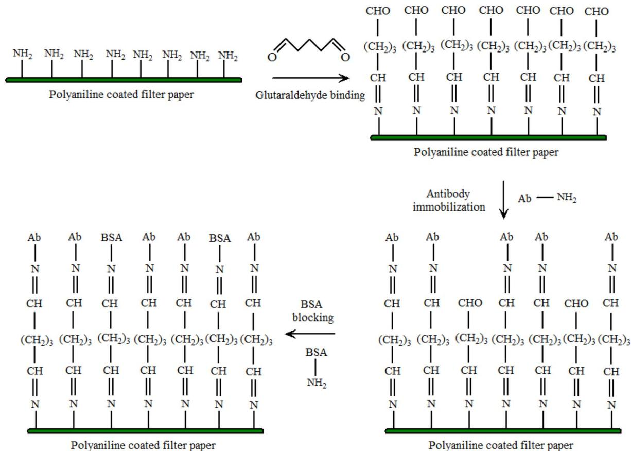
Fig. 4 Functionalization of PANI coated filter paper. The amine groups of PANI bonds with the one of the two aldehyde ( $-\text{CHO}$ ) groups of Glut. The other  $-\text{CHO}$  group is available for covalent bonding with the amine groups of the antibodies. A wash step is present between each modification step (reprinted with permission from IEEE, ref. 23 Mondal *et al.*, (2017)).
