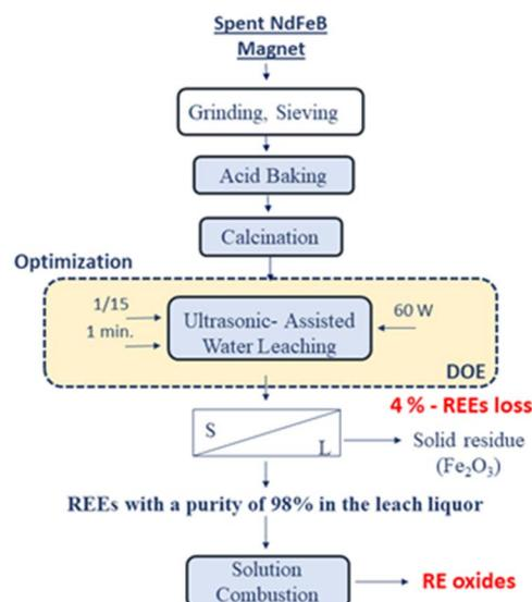
Fig. 19 The proposed conceptual flowsheet for REEs recovery from NdFeB magnets.
