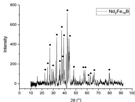
Fig. 4 X-ray diffraction analysis of NdFeB magnet powder.
