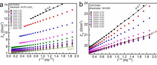
Fig. 7 Warburg factor based on the linear fits of  $Z_{re}$  against  $f^{-1/2}$  of NiO in non-aqueous Li<sup>+</sup>-based and aqueous KOH electrolytes.
