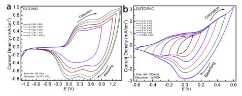
Fig. 2 (a and b) CV of NiO in 1 M LiCIO<sub>4</sub>-PC and 1 M KOH as a function of potential windows
