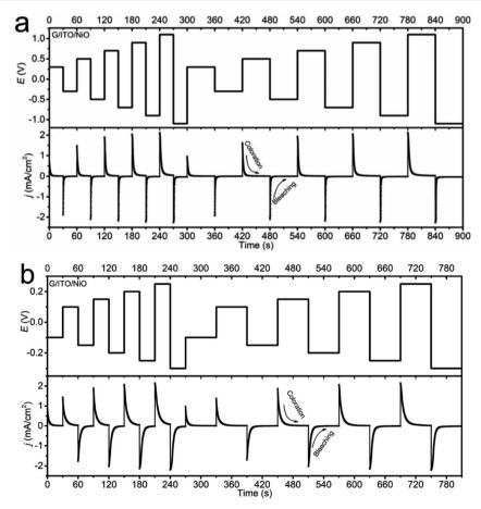
Fig. 4 MSCA response of NiO in (a) 1 M PC-LiClO<sub>4</sub> and (b) in 1 M KOH.
