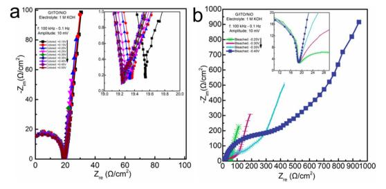
Fig. 6 EIS data and analysis for NiO thin films measured in 1 M KOH electrolyte: (a) gradual coloration applying increased magnitude potentials (+0.1 V, +0.5 V); (b) gradual bleaching range from (-0.25 V, -0.4 V).
