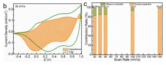
Fig. 9 (a) CV curves from 20 mV s $^{-1}$  to 150 mV s $^{-1}$  scan rates (b) CV curves at 30 mV s $^{-1}$  illustrating the surface capacitance contribution (shadowed area) to the total. (c) Percentage of diffusion-controlled and surface capacitive behavior varying with scan rate.
