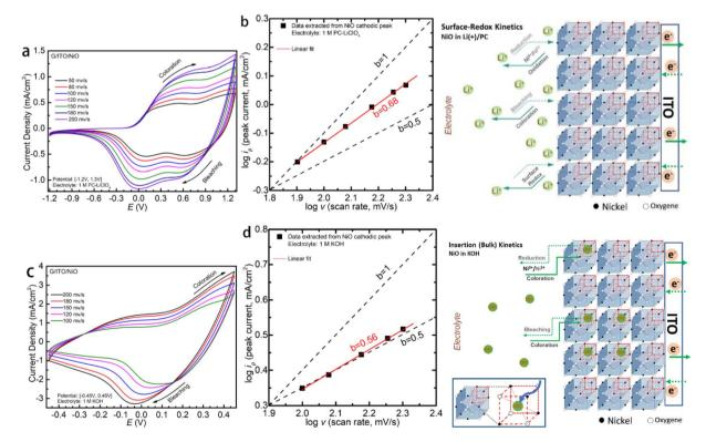
Fig. 3 (a and c) CV curves at different scan rates of NiO in Li-PC and KOH, respectively; (b and d) linear fitting of  $\log i_P vs. \log v$  and proposed dominant electrochemical kinetics at the interface in Li-PC and KOH, respectively.
