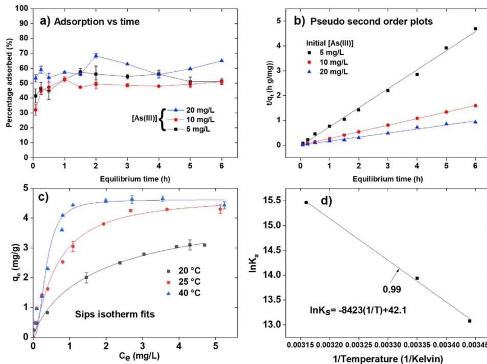
Fig. 7 (a) Adsorption vs. time; (b) pseudo 2nd order model; plots of initial As(III) concentrations of 5, 10, and 20 mg L<sup>-1</sup>; (c) the Sips isotherm fits of As(III) adsorption; and (d) van't Hoff plot of  $\ln K_s$  vs.  $1/T$  for the As(III) adsorption. Reproduced from ref. 95 with permission from Elsevier, copyright 2019.
