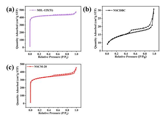
Fig. 5 Nitrogen absorption–desorption isotherms of (a) pure MIL-125(Ti), (b) NSCDBC and (c) NSCM-20.
