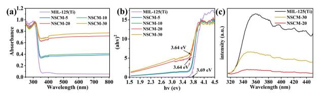
Fig. 6 (a) UV-vis absorption spectra of pure MIL-125(Ti) and different NSCDBC/MIL-125(Ti) composite materials, (b) bandgap energy of photocatalysts, (c) PL spectra of MIL-125(Ti), NSCM-20 and NSCM-30.
