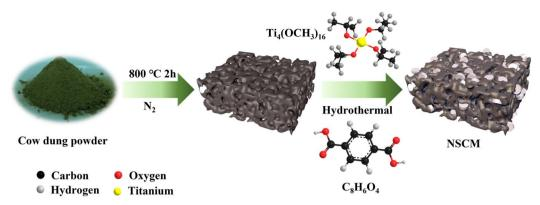
Fig. 1 Simplified flow chart for the preparation of NSCDBC/MIL-125(Ti).
