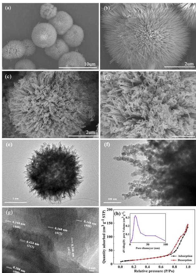
Fig. 2 SEM results of precursor (a and b) and  $\text{NiCo}_2\text{O}_4$  (c and d). TEM (e and f) and HRTEM (g) image of  $\text{NiCo}_2\text{O}_4$ . (h)  $\text{N}_2$  adsorption isotherm and the corresponding pore diameter distribution (inset) of  $\text{NiCo}_2\text{O}_4$ .
