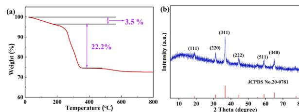
Fig. 1 (a) Thermogravimetric analysis of precursor. (b) XRD diagram of NiCo<sub>2</sub>O<sub>4</sub>.
