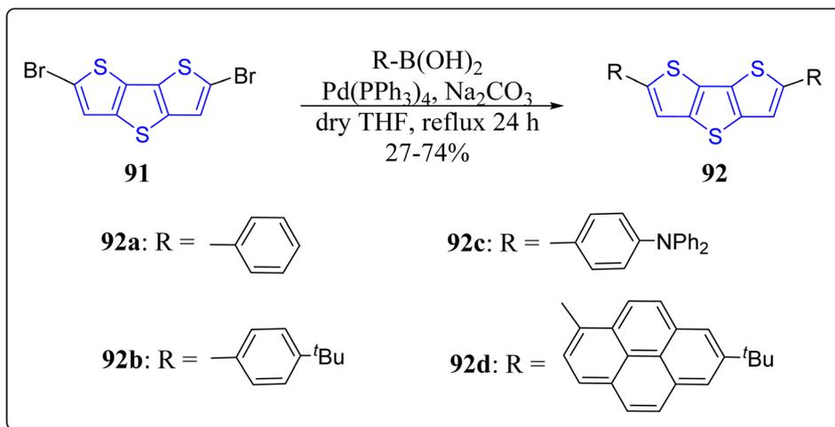
Scheme 12 Designed synthesis of D- $\pi$ -D monomers via Suzuki coupling reaction.
