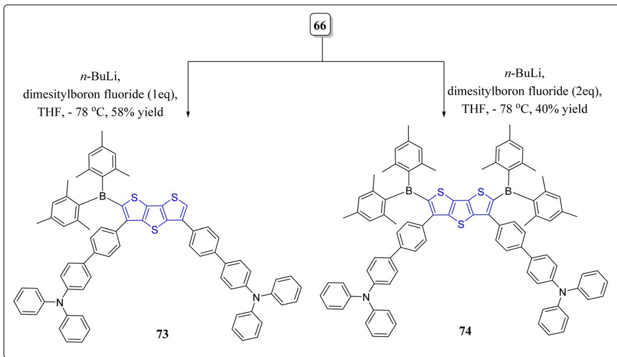
Scheme 10 Construction of the boron-based compound **73** and **74**.
