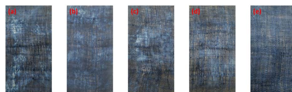
Fig. 4 Optical images of dyed grass cloth samples pre-treated with various aqueous alkali solution pick-up: (a) 60%, (b) 80%, (c) 100%, (d) 120%, and (e) 140%.
