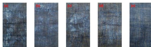
**Fig. 4** Optical images of dyed grass cloth samples pre-treated with various aqueous alkali solution pick-up: (a) 60%, (b) 80%, (c) 100%, (d) 120%, and (e) 140%.
