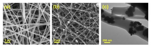
Fig. 2 SEM image of the CNF (a), SEM image (b) and TEM image (c) of the Ni<sub>3</sub>Sn<sub>2</sub>@CNF.
