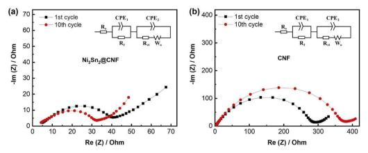
Fig. 6 Nyquist plots of the Ni<sub>3</sub>Sn<sub>2</sub>@CNF (a) and CNF (b) measured after 1st and 10th cycles. Insets: equivalent circuit models.
