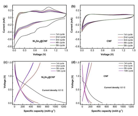
Fig. 4 CV curves of the  $Ni_3Sn_2$ @CNF (a) and CNF (b) & charge-discharge profiles of the  $Ni_3Sn_2$ @CNF (c) and CNF (d) at 0.1C.
