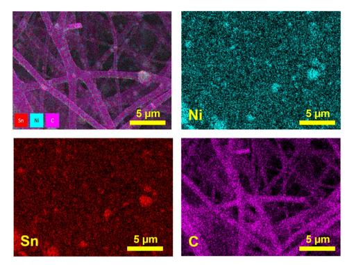
Fig. 3 Elemental mapping of the Ni<sub>3</sub>Sn<sub>2</sub>@CNF.
