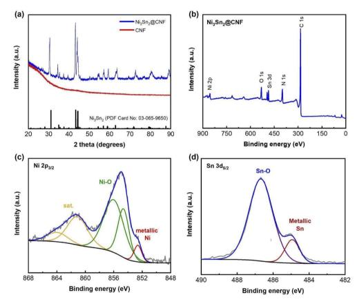
Fig. 1 XRD patterns of both  $Ni_3Sn_2@CNF$  and CNF samples (a), XPS survey spectrum (b),  $Ni\ 2p_{3/2}$  (c) and  $Sn3d_{5/2}$  (d) XPS spectra of the  $Ni_3Sn_2@CNF$ .
