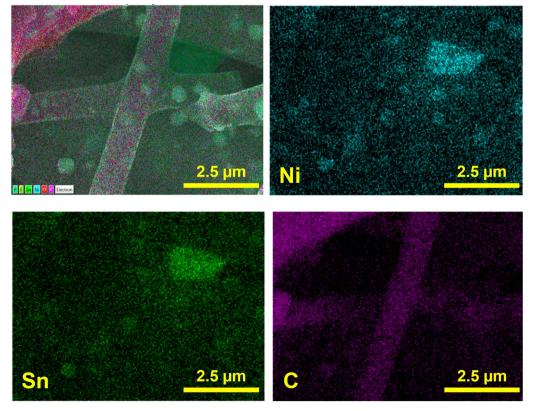
Fig. 7 Elemental mapping of the Ni<sub>3</sub>Sn<sub>2</sub>@CNF after 70 cycles at 0.1C.
