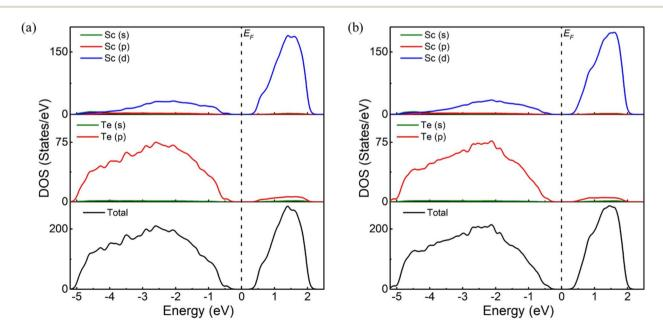
Fig. 6 The total and partial density of states (DOSs). (a) DOSs of amorphous  $Sc_2Te_3$  at 300 K and (b) DOSs of supercooled  $Sc_2Te_3$  at 773K, using the mBJLDA functional. The dashed vertical line is the Fermi level ( $E_F$ ), corresponding to the zero point energy.
