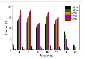
Fig. 4 The distribution of medium-range-order (MRO) in the  $Sc_2Te_3$  system at different temperatures.
