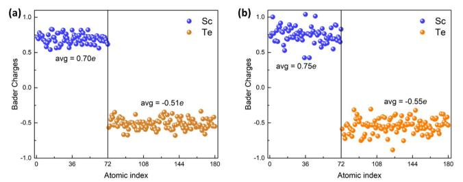
Fig. 7 Bader charge distributions for an 180-atom  $Sc_2Te_3$  system. (a) Bader charges of amorphous  $Sc_2Te_3$  at 300 K and (b) Bader charges of supercooled  $Sc_2Te_3$  at 773 K. Blue and orange dots represent 72 Sb and 120 Te atoms. The average values are given for both atomic species.
