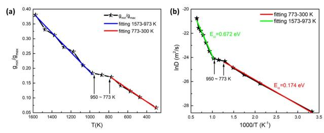
Fig. 5 (a) The calculated Wendt–Abraham parameter of the  $Sc_2Te_3$  system as a function of temperature. (b) The diffusion coefficient (*D*) of the  $Sc_2Te_3$  system at different temperatures. The blue and green solid lines are the linear fitting results from 1573 to 973 K, while the red solid lines are the linear fitting results from 773 to 300 K.
