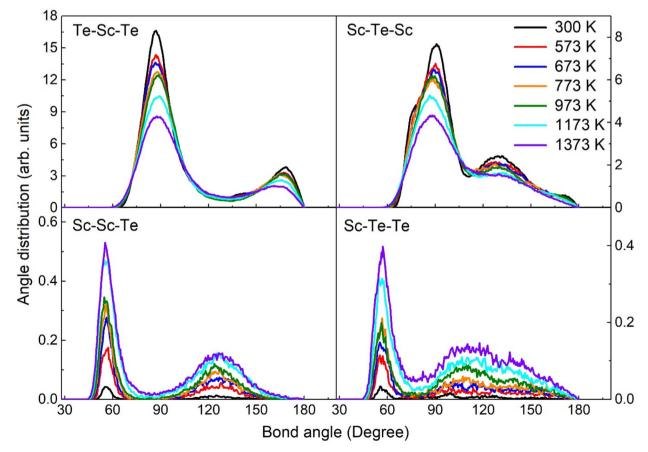
Fig. 3 The calculated partial angular distribution function (ADF) of the Sc<sub>2</sub>Te<sub>3</sub> system at different temperatures.
