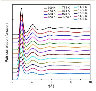
Fig. 1 The total pair-correlation functions (PCF) of the  $Sc_2Te_3$  system at different temperatures. Note that, for clarity, each curve has been vertically displaced from the curve below.
