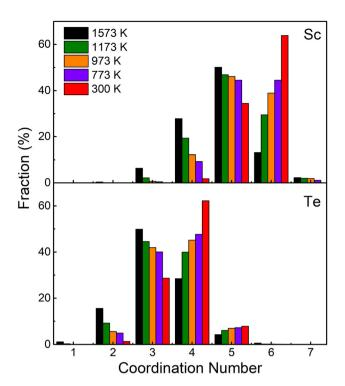
Fig. 2 The coordination number (CN) distributions for the Sc- and Tecentered atoms in the  $Sc_2Te_3$  system at different temperatures.
