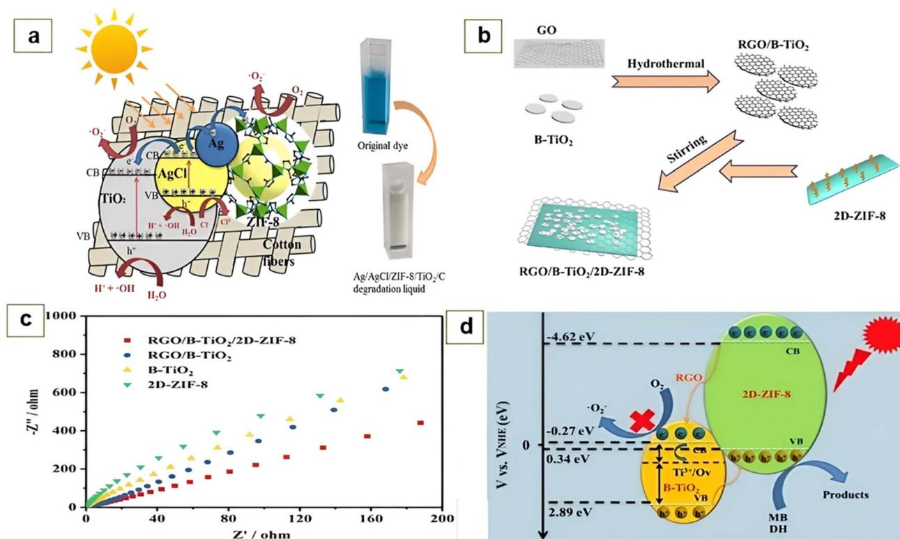
Fig. 6 (a) Photo-degradation mechanism of MB with Ag/AgCl/ZIF-8/TiO<sub>2</sub>/C hybrid. Reproduced from ref. 126 Copyright 2019, Springer. (b) Process for the elaboration of the ternary system RGO/B-TiO<sub>2</sub>/2D-ZIF-8. (c) EIS analysis of B-TiO<sub>2</sub>, RGO/B-TiO<sub>2</sub>, 2D-ZIF-8 and RGO/B-TiO<sub>2</sub>/2D-ZIF-8. (d) Photo-degradation mechanism of MB with RGO/B-TiO<sub>2</sub>/2D-ZIF-8 ternary system. Reproduced with permission from ref. 127 Copyright ©2020, Wiley VCH.
