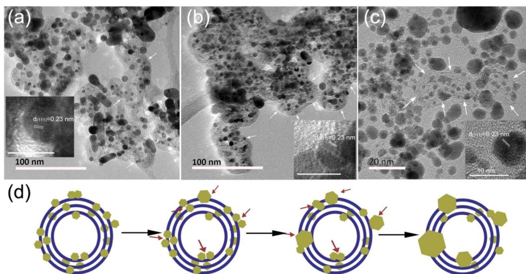
Fig. 8 TEM images of the Pt/C catalyst after 1800 h practical application (cathode (a) and anode (b)), and after heating at 600 °C in the *in situ* DENSolutions climate air holder (c). By comparing the changes in the Pt/C catalysts under the two conditions, a schematic illustration of Pt particle growth (d).
