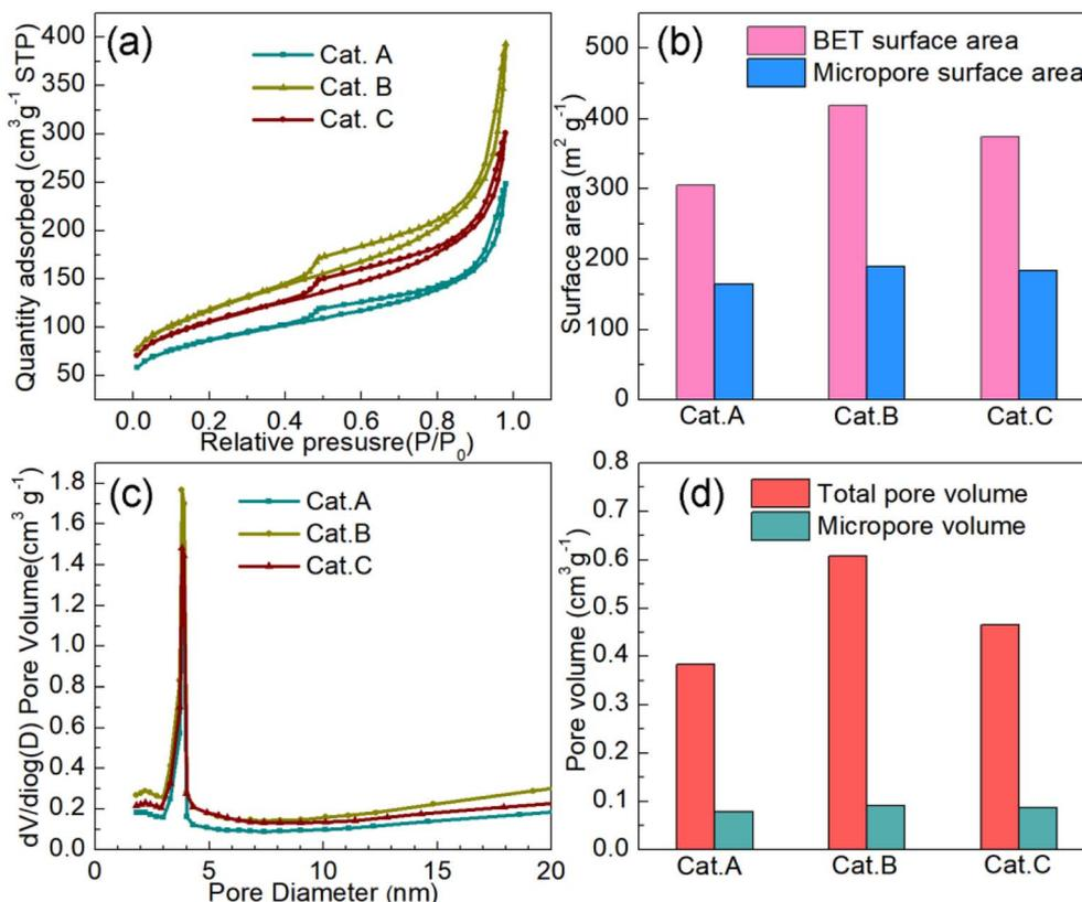
Fig. 1 (a)  $N_2$  adsorption-desorption isotherms of three commercial catalysts. Summary of their specific surface area (b), pore size distribution (c) and pore volume (d).
