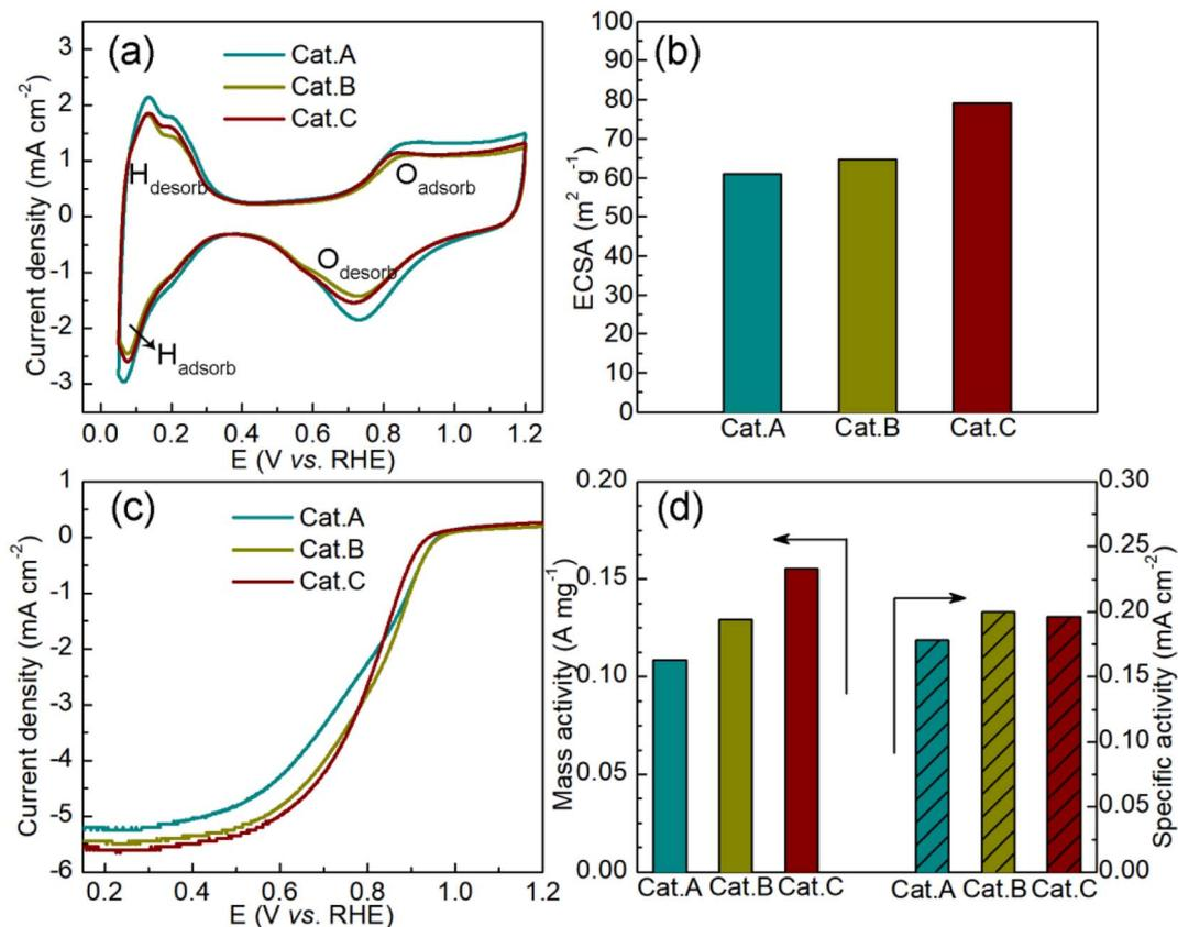
Fig. 5 (a) CV curves of the three commercial Pt/C catalysts and (b) corresponding ECSA, (c) LCV curves of the ORR reaction in 0.1 mol L<sup>-1</sup> HClO<sub>4</sub> and (d) the corresponding mass activities and specific activities.
