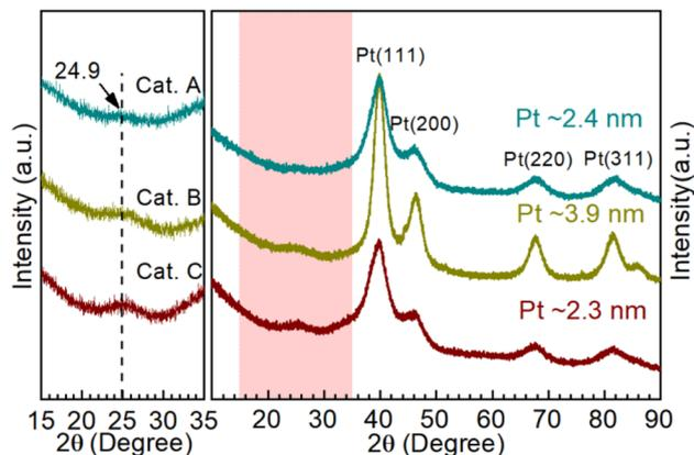
Fig. 3 XRD patterns of Cat.A, Cat.B and Cat.C, where the light pink area is enlarged to clearly show the structural information of the carbon supports and the average grain size (Cat.A:  $\sim$ 2.4 nm, Cat.B:  $\sim$ 3.9 nm, and Cat.C:  $\sim$ 2.3 nm) was calculated according to the Scherrer formula.
