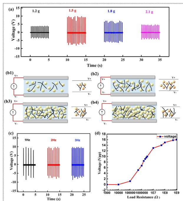
Fig. 6 (a) Time dependent output voltage ( $V_{oc}$ ) of the PENG device at various weights of PZT (1.2, 1.5, 1.8, and 2.1 g). (b1–b4) Schematic representation of the PENG with different amounts of the added ceramic and MWCNTs load concentration. (c) Output voltage ( $V_{oc}$ ) of the PENG device at different frequencies. (d) Effect of external load resistance on the output of the PENG device.
