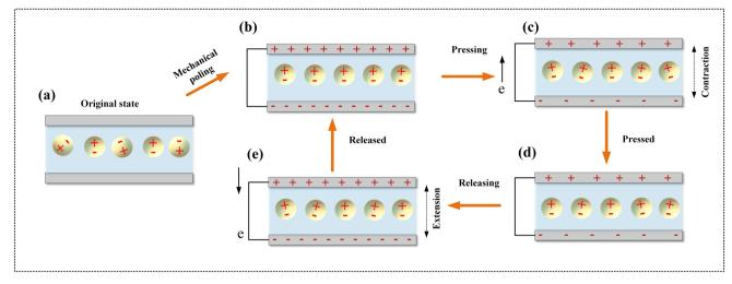
Fig. 4 Schematic representation of the PENG working mechanism. (a) Original state of dipoles in the absence of external mechanical poling, (b) the dipoles are aligned in the same direction after the mechanical poling process, (c) the piezoelectric voltage is generated by applying compressive force, (d) maximized press state with highest polarization density, (e) dipoles are back facing the opposite direction as the compressive force is released.
