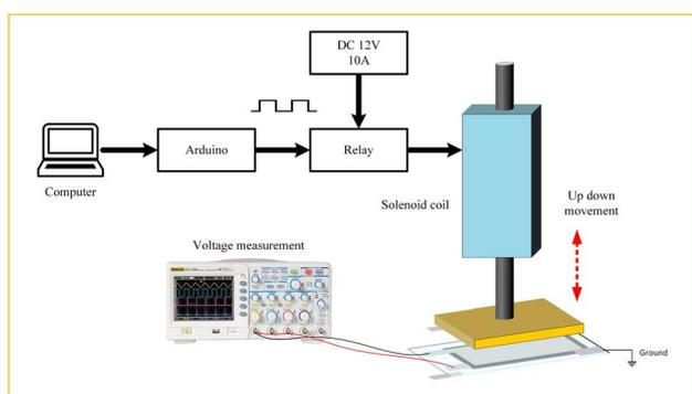
Fig. 5 Schematic of the energy harvesting measurement setup.
