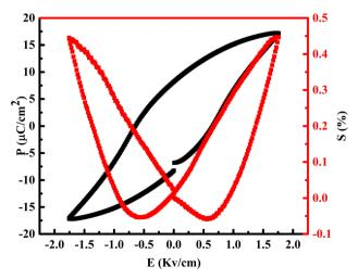
Fig. 3 Electric field dependent P-E and S-E loops.
