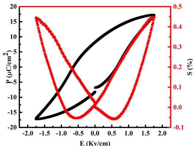
Fig. 3 Electric field dependent P–E and S–E loops.
