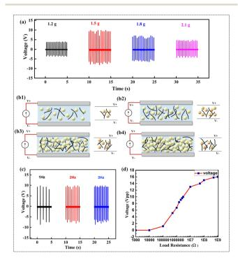
Fig. 6 (a) Time dependent output voltage ( $V_{\rm oc}$ ) of the PENG device at various weights of PZT (1.2, 1.5, 1.8, and 2.1 g). (b1-b4) Schematic representation of the PENG with different amounts of the added ceramic and MWCNTs load concentration. (c) Output voltage ( $V_{\rm oc}$ ) of the PENG device at different frequencies. (d) Effect of external load resistance on the output of the PENG device.
