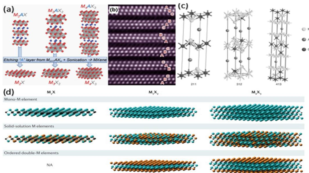
**Fig. 1** (a) MAX phases 211, 312 and 413 crystal structures. (b) STEM-HAADF picture of a  $Ti_3C_2T_x$  grain in the (120) zone-axis orientation. (c) Crystal structure of the  $M_3AX_2$  phase with the  $P6_3/mmc$  space group. (d) Mono-transition metal MXene, Solid solution-transition metal MXene, ordered-double MXene.<sup>20,21,23,24</sup>
