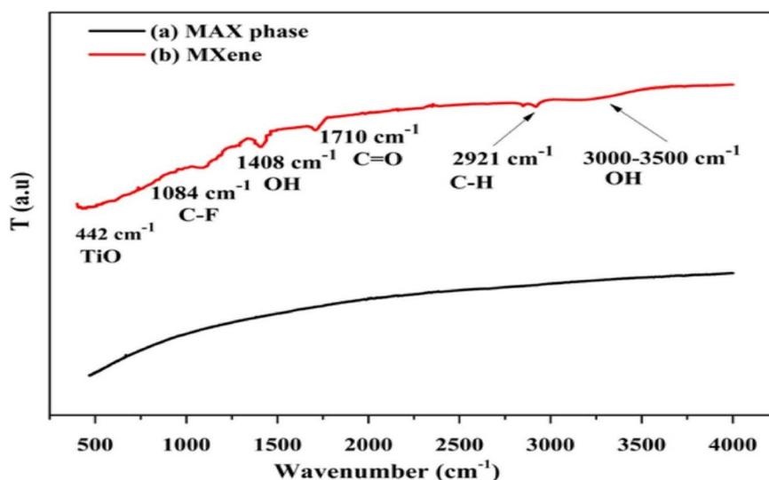
Fig. 3 FTIR spectra of (a) MAX phase (b) MXene.<sup>34</sup>
