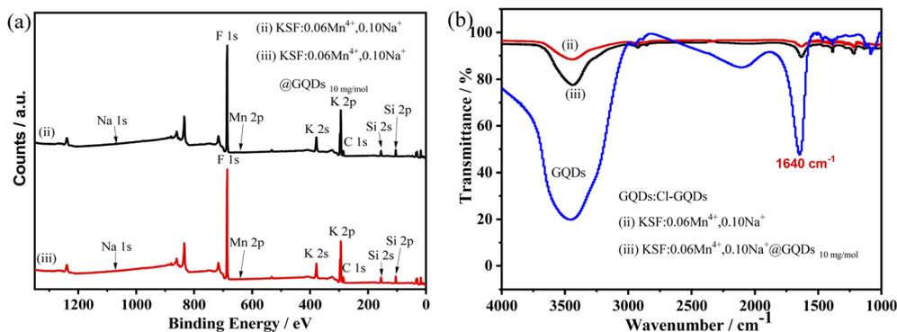
Fig. 2 XPS and FTIR spectra of samples, (ii) KSF: 0.06Mn<sup>4+</sup>, 0.10Na<sup>+</sup>, and (iii) KSF: 0.06Mn<sup>4+</sup>, 0.10Na<sup>+</sup> @ GQDs 10 mg mol<sup>-1</sup> (a) XPS spectra, (b) FTIR spectra.
