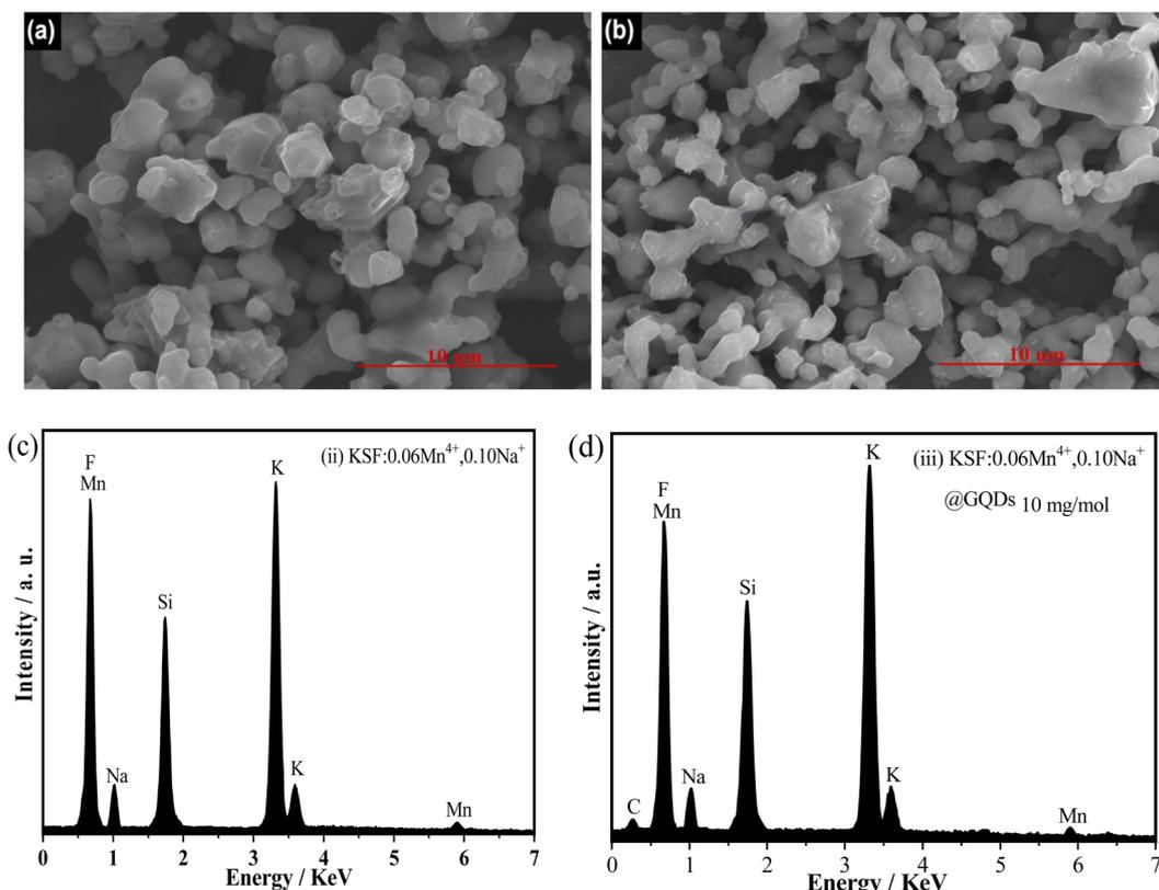
Fig. 3 SEM images and EDS spectra of two samples, (ii) KSF: 0.06Mn<sup>4+</sup>, 0.10Na<sup>+</sup> and (iii) KSF: 0.06Mn<sup>4+</sup>, 0.10Na<sup>+</sup> @ GQDs 10 mg mol<sup>-1</sup>: (a and b) SEM images of sample (ii) and (iii) (c and d) EDS spectra.
