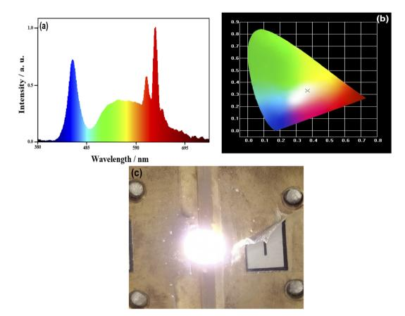
Fig. 8 Performances of prototype WLEDs using the mixing phosphors of KSF:  $0.06 \text{Mn}^{4+}$ ,  $0.10 \text{Na}^+$  @ GQDs 10 mg mol<sup>-1</sup> and YAG:  $\text{Ce}^{3+}$  based on InGaN chip under a 20 mA drive current: (a) Electroluminescence spectra, (b) CIE chromaticity diagram, (c) A photograph of the white emission spectrum of the driven LED.
