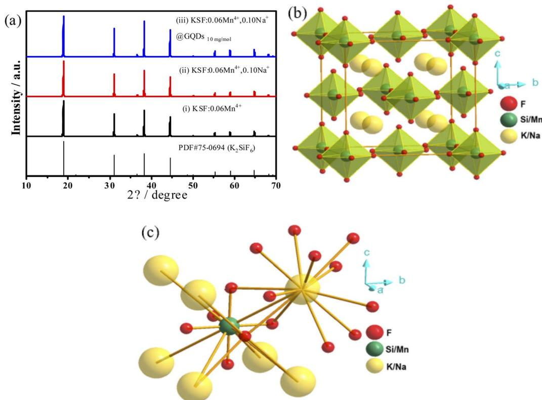
Fig. 1 (a) XRD patterns of the three samples: (i) KSF: 0.06Mn<sup>4+</sup>, (ii) KSF: 0.06Mn<sup>4+</sup>, 0.10Na<sup>+</sup>, (iii) KSF: 0.06Mn<sup>4+</sup>, 0.10Na<sup>+</sup> @ GQDs 10 mg mol<sup>-1</sup>, (b) The built unit cell structure of the sample (ii), (c) coordination environment surrounding Si/Mn.
