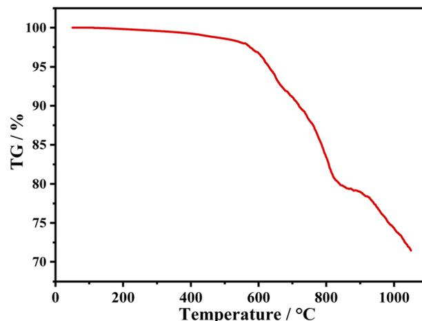
Fig. 7 TG of sample, (iii) KSF: 0.06Mn<sup>4+</sup>, 0.10Na<sup>+</sup> @ GQDs 10 mg mol<sup>-1</sup>.
