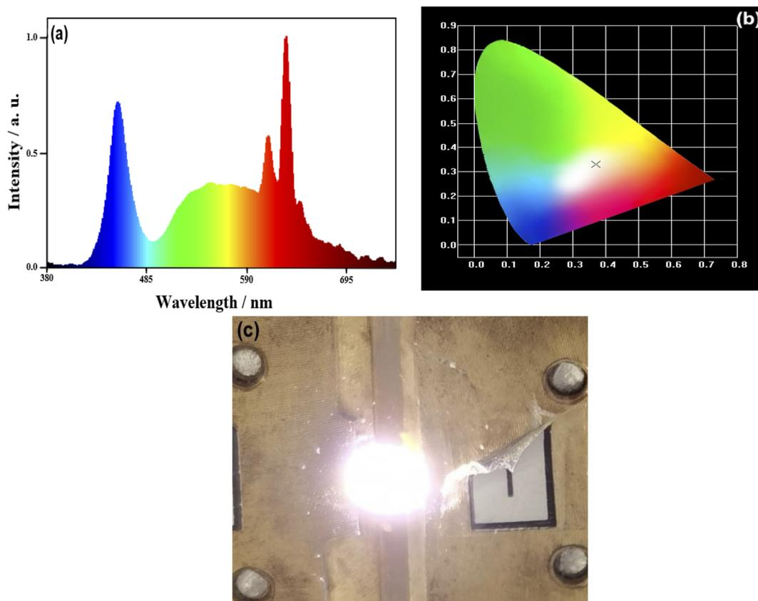
Fig. 8 Performances of prototype WLEDs using the mixing phosphors of KSF:  $0.06\text{Mn}^{4+}$ ,  $0.10\text{Na}^+$  @ GQDs  $10\text{ mg mol}^{-1}$  and YAG :  $\text{Ce}^{3+}$  based on InGaN chip under a 20 mA drive current: (a) Electroluminescence spectra, (b) CIE chromaticity diagram, (c) A photograph of the white emission spectrum of the driven LED.
