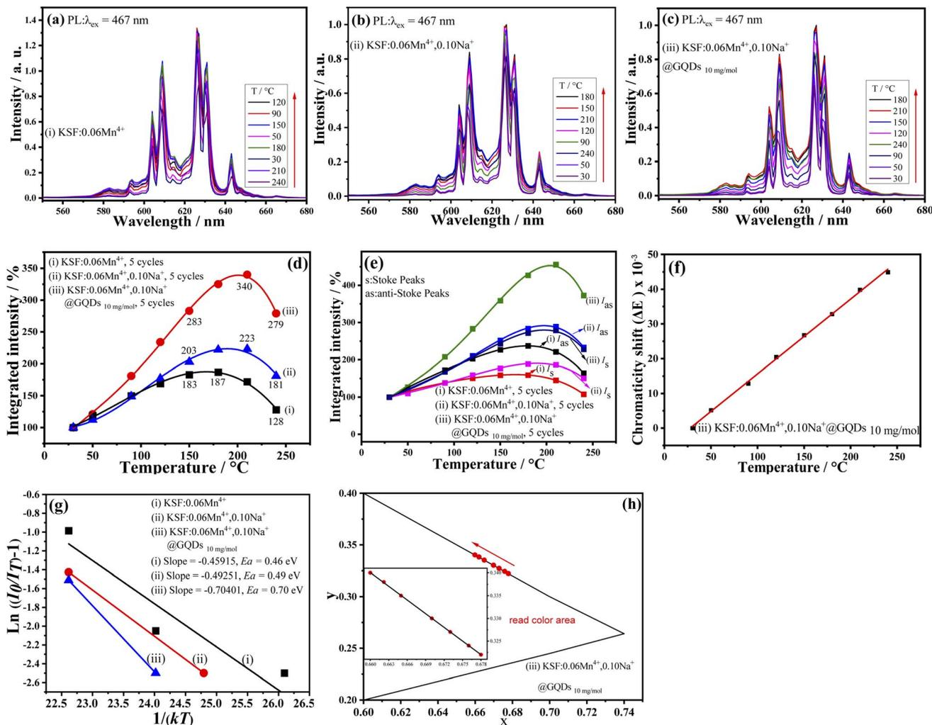
Fig. 6 Temperature-dependent PL performances of three samples, (i) KSF: 0.06Mn<sup>4+</sup>, (ii) KSF: 0.06Mn<sup>4+</sup>, 0.10Na<sup>+</sup>, (iii) KSF: 0.06Mn<sup>4+</sup>, 0.10Na<sup>+</sup> @ GQDs 10 mg mol<sup>-1</sup>: (a) and (b) and (c) PL spectra; (d) Integrated intensity curves; (e) Integrated intensity curves of Stoke and anti-Stoke peaks, (f) Chromaticity shift of sample (iii), (g)  $E_a$  curves, (h) CIE color coordinates of sample (iii).
