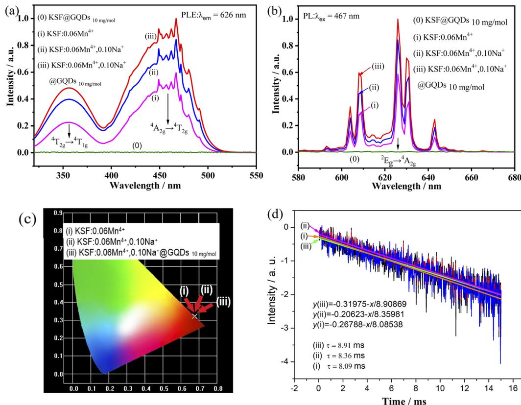
Fig. 4 Luminescent properties of four samples, (0) KSF @ GQDs 10 mg mol<sup>-1</sup>, (i) KSF: 0.06Mn<sup>4+</sup>, (ii) KSF: 0.06Mn<sup>4+</sup>, 0.10Na<sup>+</sup>, (iii) KSF: 0.06Mn<sup>4+</sup>, 0.10Na<sup>+</sup> @ GQDs 10 mg mol<sup>-1</sup>: (a) and (b) PLE and PL spectra, (c) CIE chromaticity diagram, (d) Lifetime curves of the samples (i–iii).
