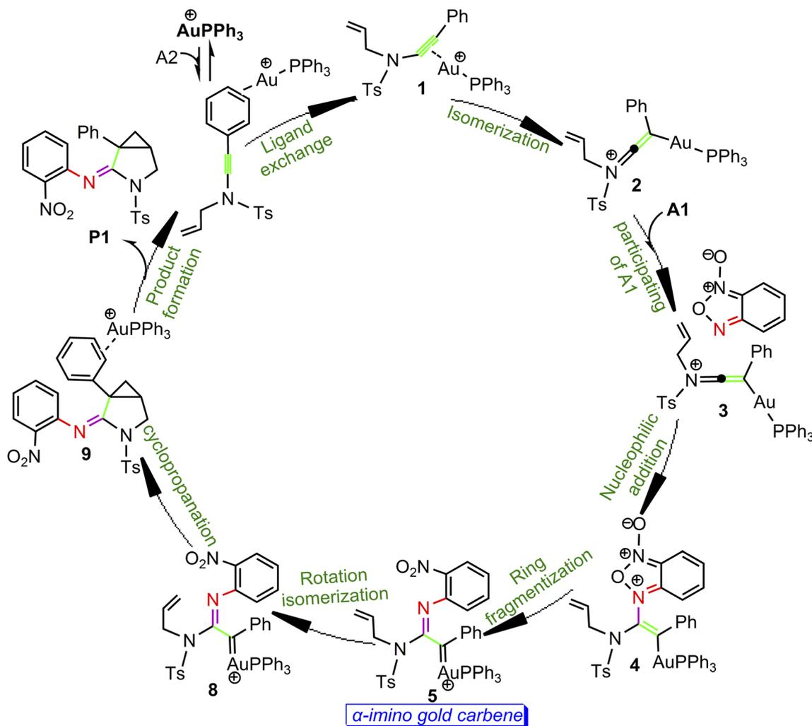
Scheme 5 Catalytic cycle derived from DFT calculations.
