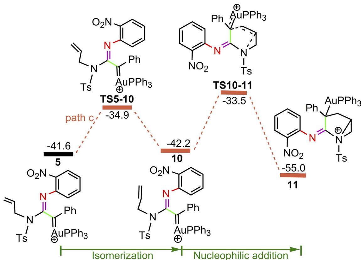
Fig. 4 Potential energy surface in PhCl solvent for the other pathway of nucleophilic attacks on  $\alpha$ -imino gold carbene **5**. The solvent-corrected relative free energies are given in kcal mol<sup>-1</sup>.
